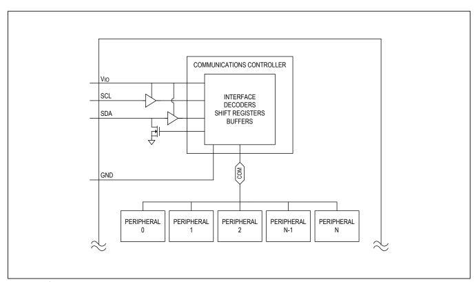
Figure 22. I<sup>2</sup>C Simplified Block Diagram
