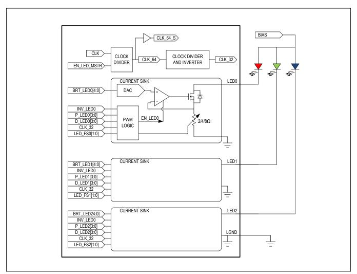
Figure 21. Current Sink Block Diagram
