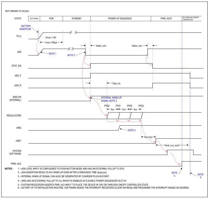
Figure 7. Startup Timing Diagram Due to nEN
