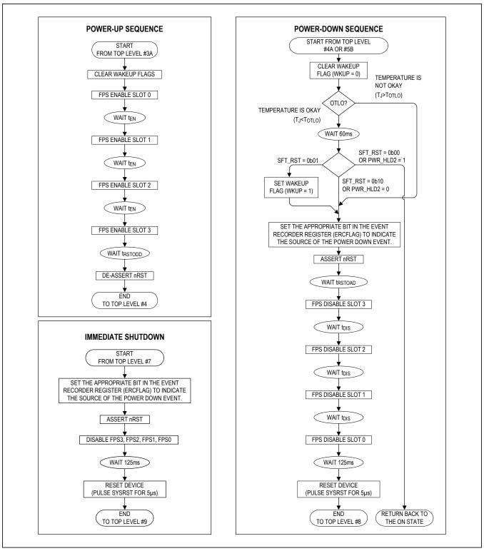
Figure 5. Power-Up/Power-Down Sequence
