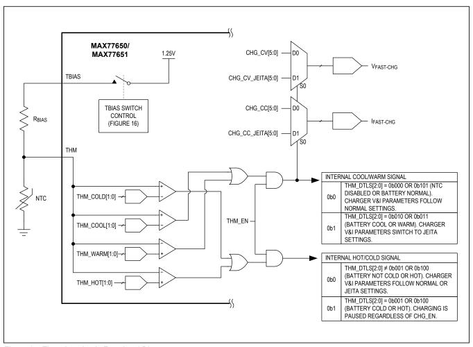
Figure 14. Thermistor Logic Functional Diagram
