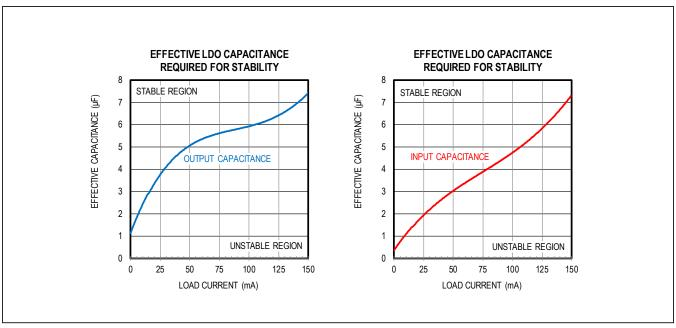
Figure 19. LDO Capacitance for Stability
