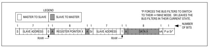
Figure 29. Reading from a Single Register with the Read Byte Protocol
