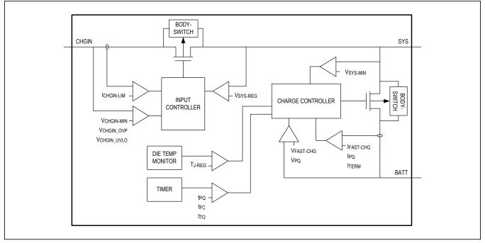
Figure 11. Charger Simplified Control Loops
