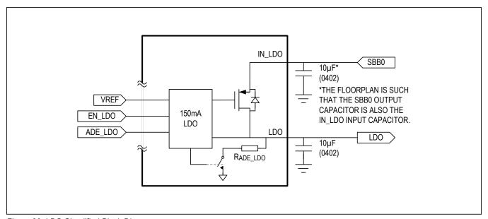
Figure 20. LDO Simplified Block Diagram
