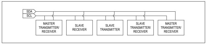
Figure 23. I<sup>2</sup>C System Configuration
