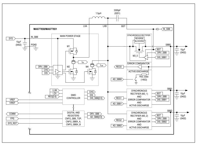
Figure 18. SIMO Detailed Block Diagram
