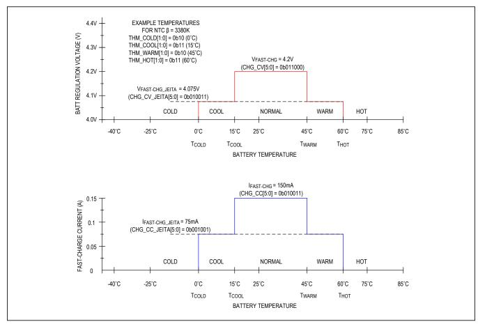
Figure 15. Safe-Charging Profile Example
