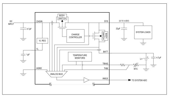
Figure 10. Linear Charger Simplified Block Diagram
