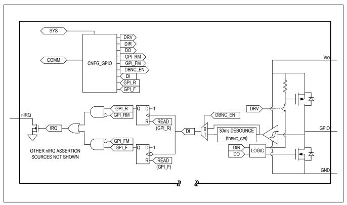
Figure 3. GPIO Block Diagram
