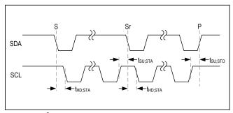
Figure 24. I<sup>2</sup>C Start and Stop Conditions
