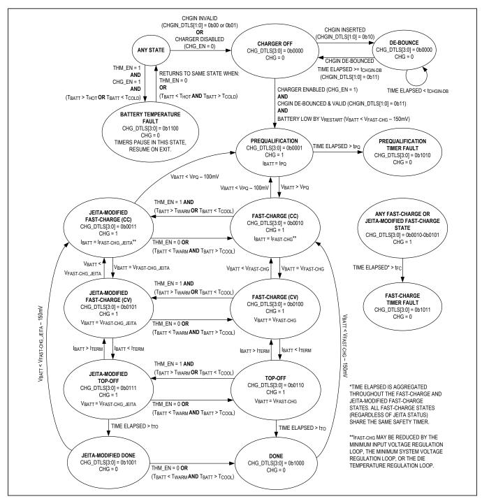
Figure 12. Charger State Diagram
