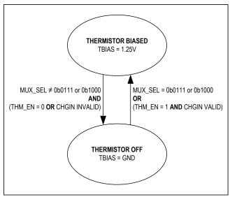
Figure 16. Thermistor Bias State Diagram
