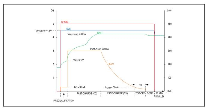
Figure 13. Example Battery Charge Profile
