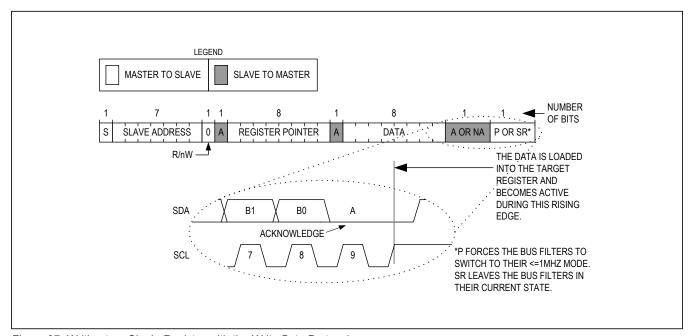
Figure 27. Writing to a Single Register with the Write Byte Protocol
