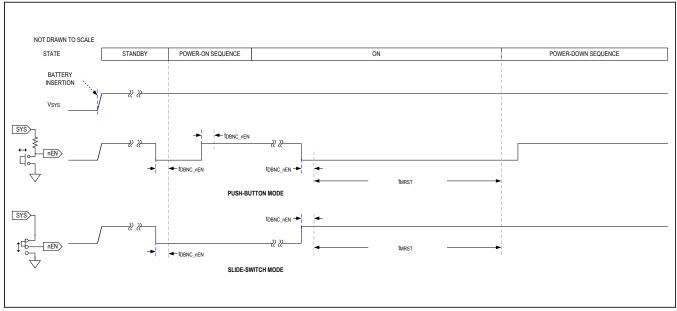
Figure 2. nEN Usage Timing Diagram
