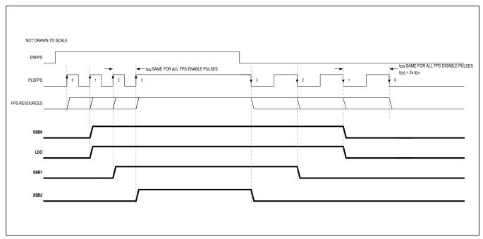
Figure 6. Flexible Power Sequencer Basic Timing Diagram
