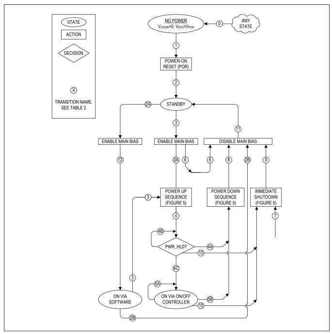
Figure 4. Top-Level On/Off Controller
