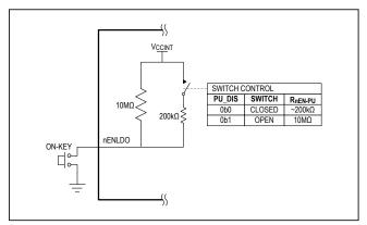
Figure 4. nENLDO Pullup Resistor Configuration
