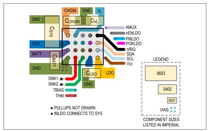
Figure 15. PCB Top-Metal and Component Layout Example
