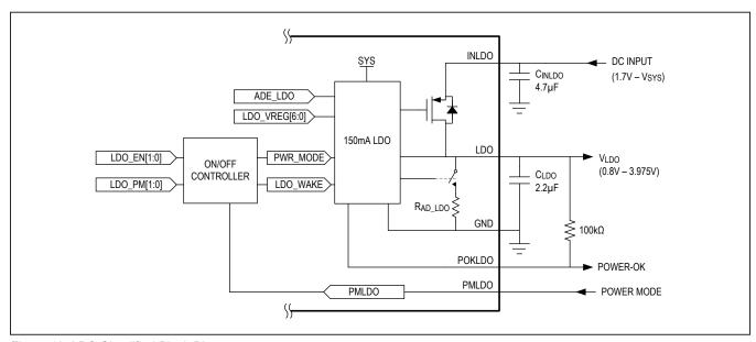
Figure 13. LDO Simplified Block Diagram
