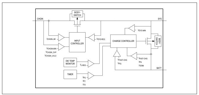
Figure 6. Charger Simplified Control Loops
