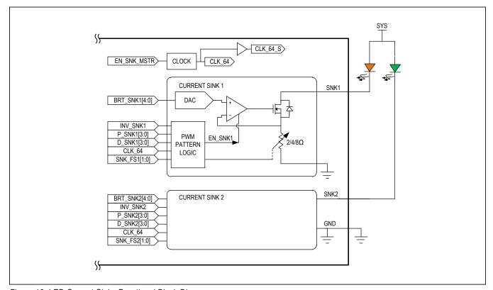
Figure 16. LED Current Sinks Functional Block Diagram
