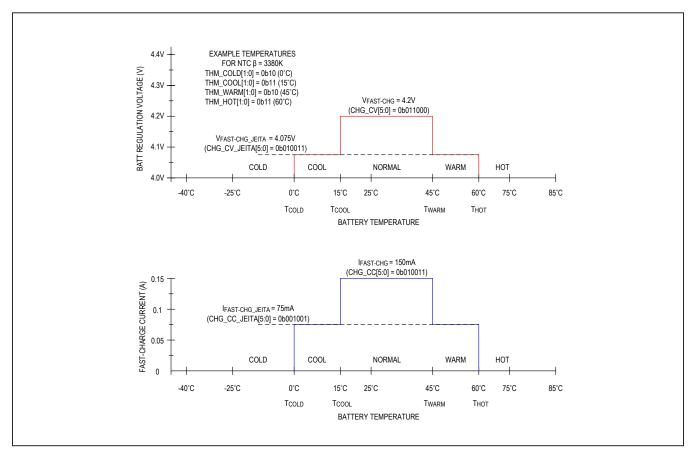
Figure 10. Safe-Charging Profile Example
