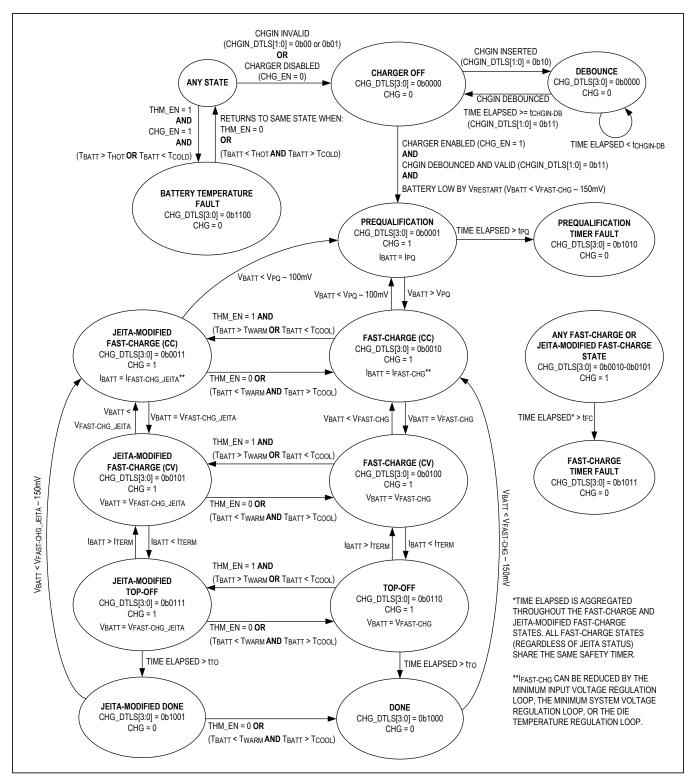
Figure 7. Charger State Diagram
