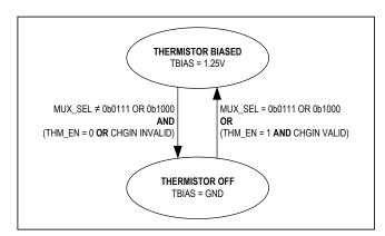
Figure 11. Thermistor Bias State Diagram
