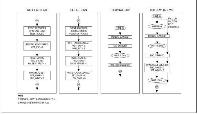
Figure 2. On/Off Controller Action Sequences
