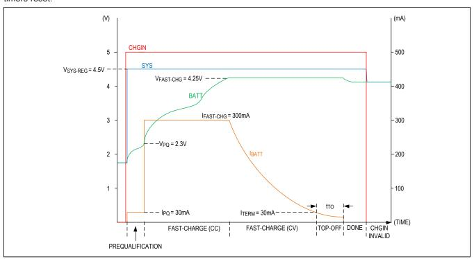
Figure 8. Example Battery Charge Profile
