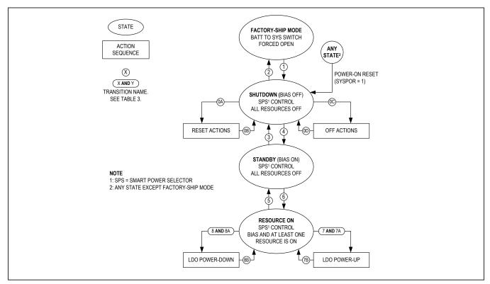
Figure 1. On/Off Controller State Machine
