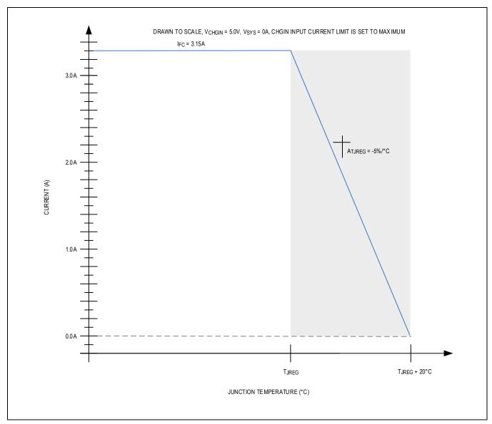
Figure 7. Charge Currents vs. Junction Temperature
