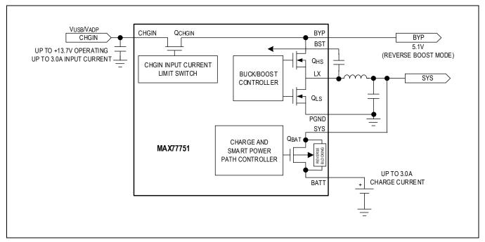
Figure 1. Simplified Functional Diagram
