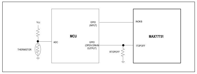
Figure 12. System Configuration for Temperature Management
