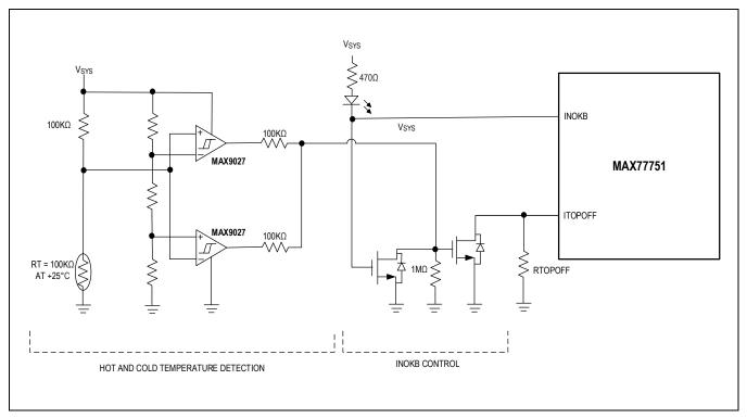
Figure 13. System Configuration for Temperature Management
