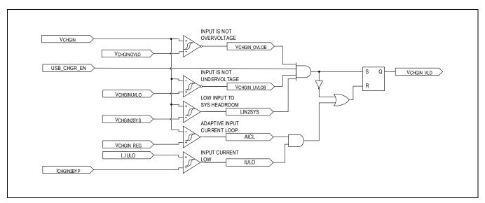
Figure 3. CHGIN Valid Signal Generation Logic
