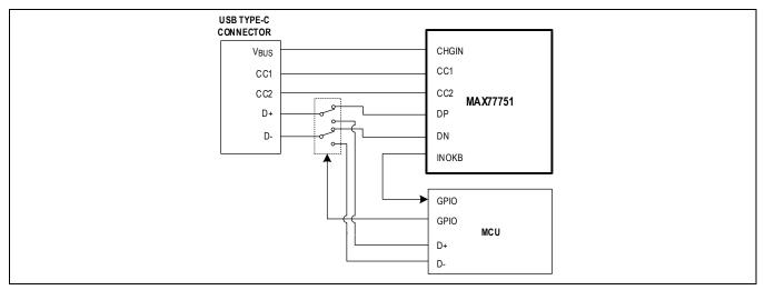
Figure 11. D+/D- Connections in a Reference System
