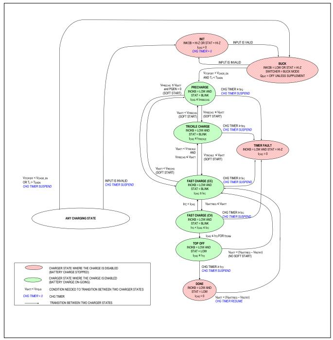
Figure 6. Charger State Diagram
