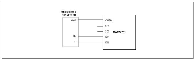
Figure 8. USB Signal Connections for a Micro-B Connector
