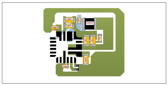
Figure 14. Recommended Placement and Layout
