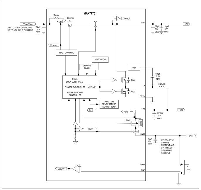
Figure 2. Battery Charger Detailed Functional Diagram
