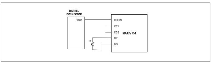
Figure 10. Connections for a Barrel Connector (1.5A Power Source)
