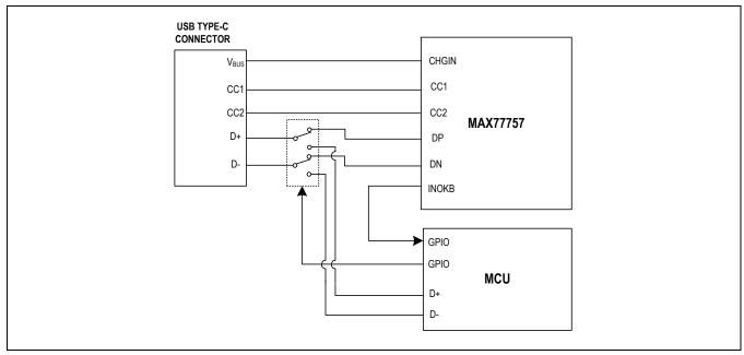
Figure 12. D+/D- Connections in a Reference System
