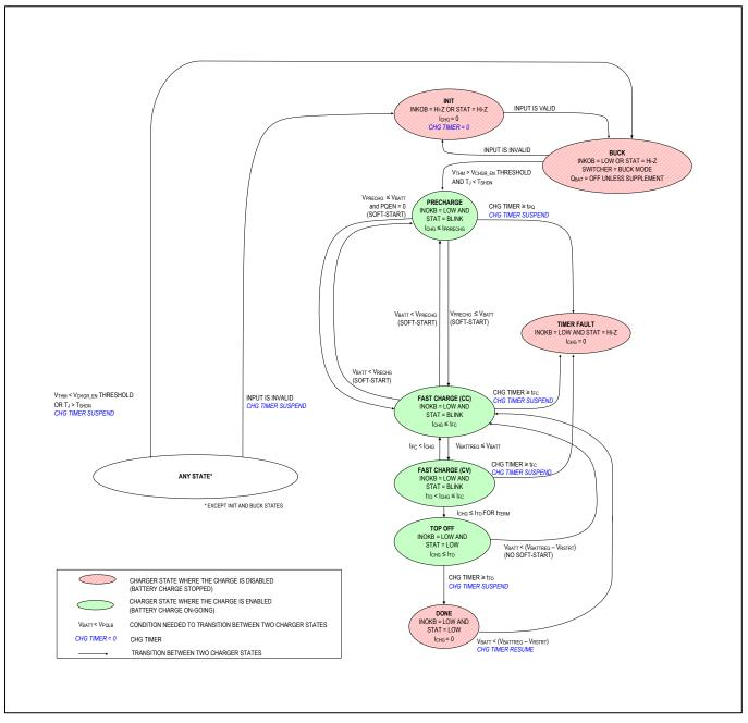
Figure 8. LiFePO4 State Machine
