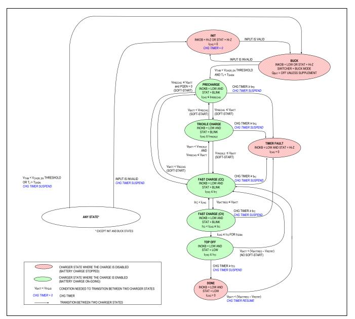
Figure 6. Li+/Li-Poly Charger State Diagram
