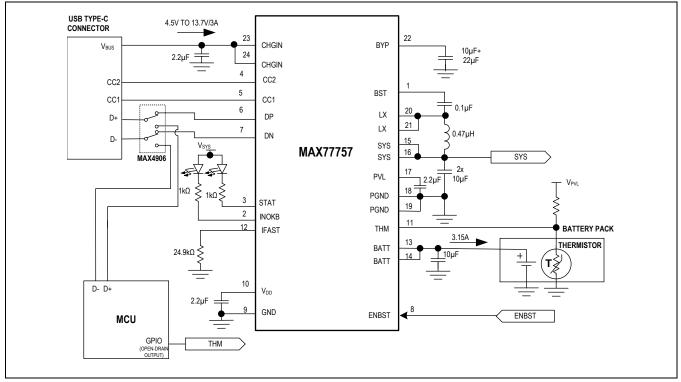
Figure 14. Typical Application Circuit
