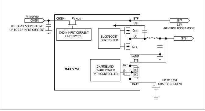
Figure 1. Simplified Functional Diagram
