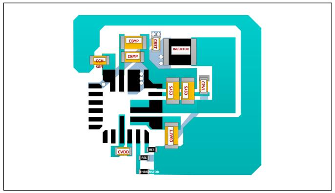
Figure 13. Recommended Placement and Layout
