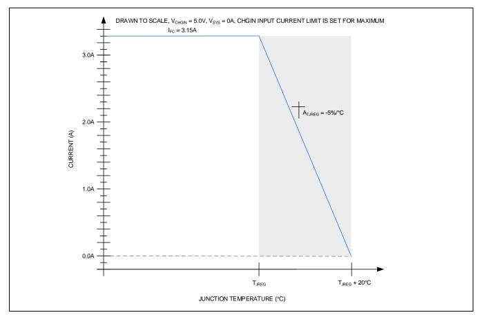
Figure 9. Charge Currents vs. Junction Temperature
