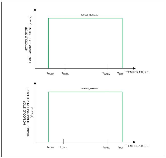
Figure 10. MAX77757H Version Hot/Cold Stop
