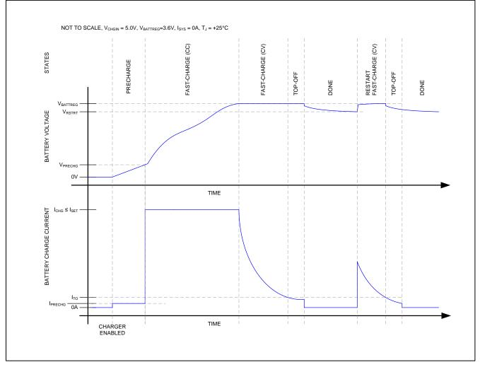
Figure 7. LiFePO<sub>4</sub> Battery Charge Profile
