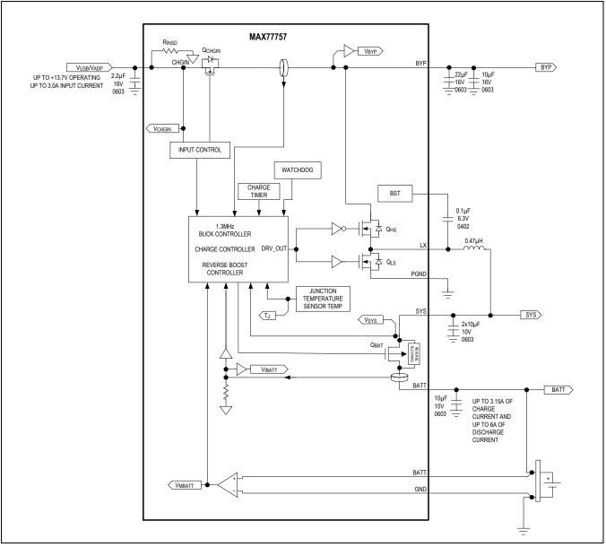
Figure 2. Main Battery Charger Detailed Functional Diagram
