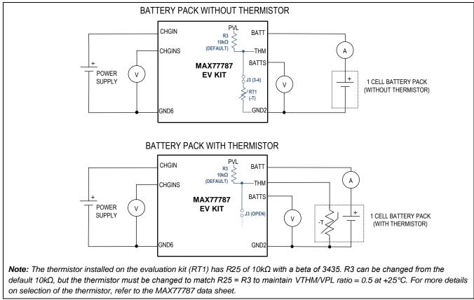
Figure 3. Battery Charger Test with Real Battery Pack
