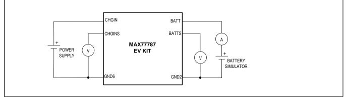
Figure 4. Battery Charger Test with Battery Simulator
