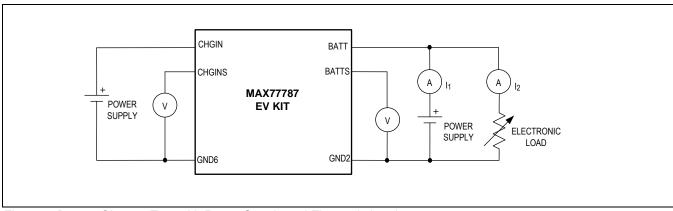
Figure 5. Battery Charger Test with Power Supply and Electronic Load
