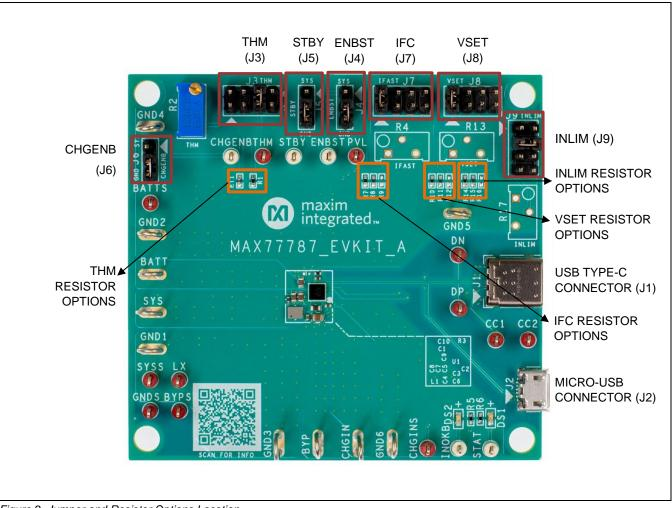
Figure 2. Jumper and Resistor Options Location
