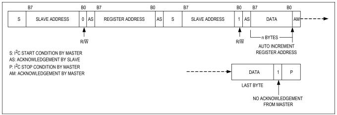
Figure 17. Master Read Operation with Register Addresses
