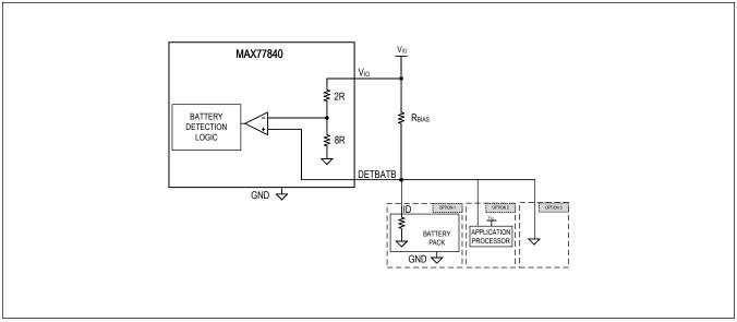
Figure 10. Battery Present Detection Circuit
