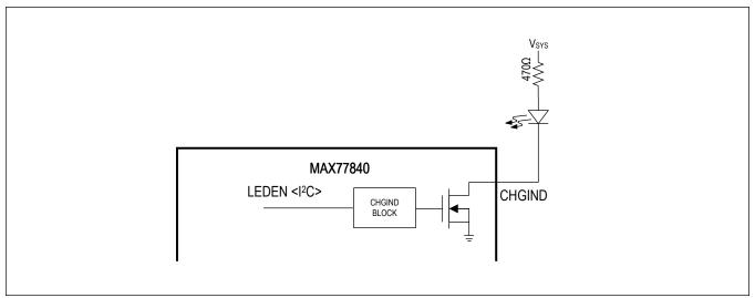
Figure 9. Charging Indicator Circuit
