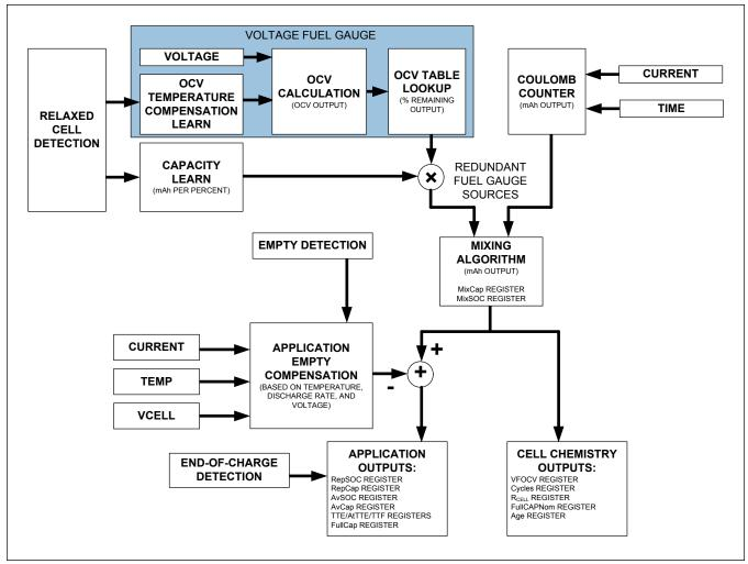
Figure 20. ModelGauge m5 Block Diagram
