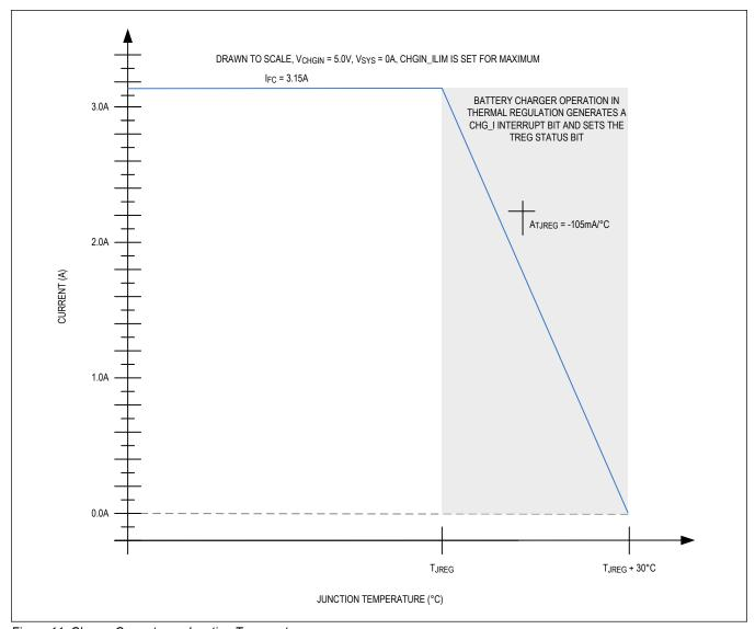
Figure 11. Charge Currents vs. Junction Temperature
