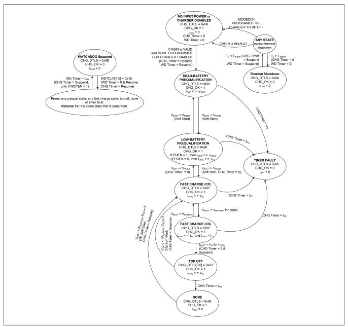
Figure 3. MAX77840 Charger State Diagram
