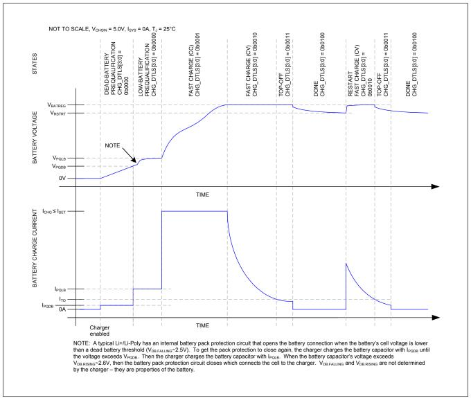
Figure 2. MAX77840 Typical Charging Profile
