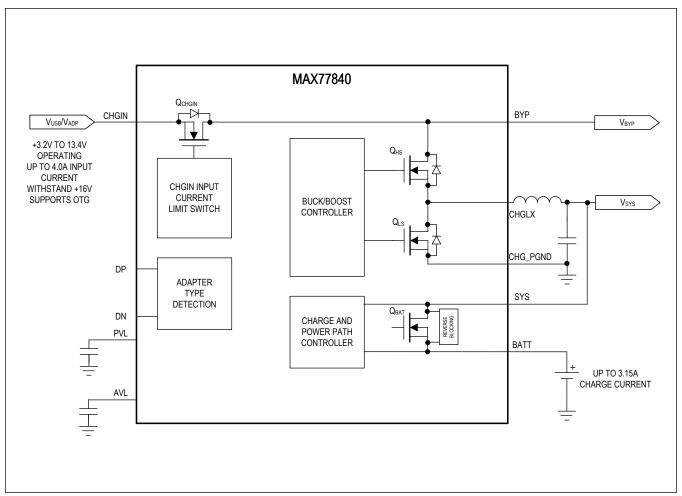
Figure 1. Switching Charger Block Diagram
