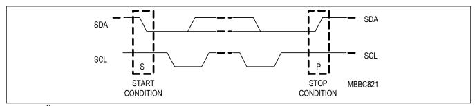
Figure 14. I<sup>2</sup>C Start and Stop
