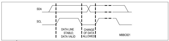
Figure 13. I<sup>2</sup>C Bit Transfer
