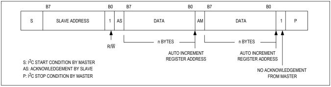
Figure 18. Master Read Operation without Register Address
