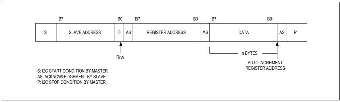
Figure 16. Master Write Operation
