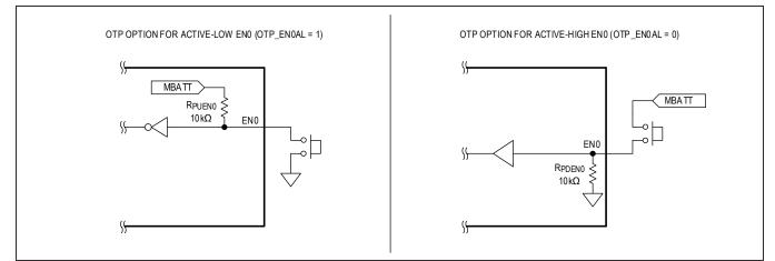
Figure 20. EN0 Simplified Input Stage: Active-High or Low
