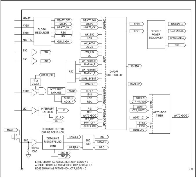
Figure 18. Simplified Block Diagram: ON/OFF Controller
