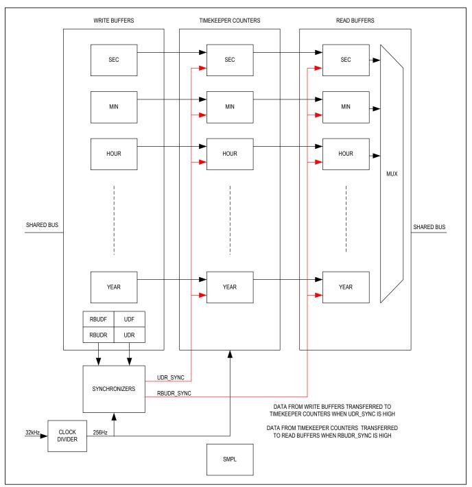
Figure 13. RTC Simplified Functional Diagram
