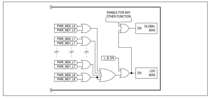
Figure 11. LDO Bias Enable Circuitry
