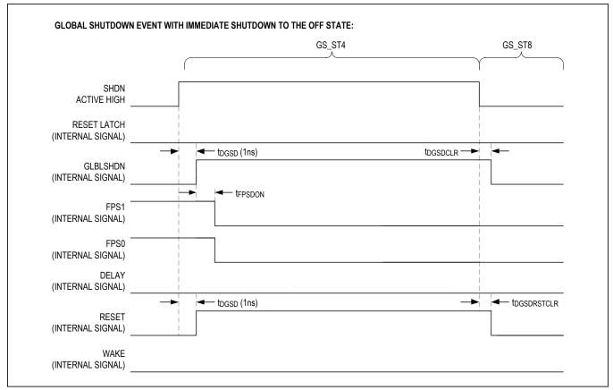
Figure 7. Simplified Timing Diagram for Global Shutdown
