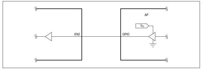
Figure 22. EN2 Simplified Input Stage: Active-High or Low
