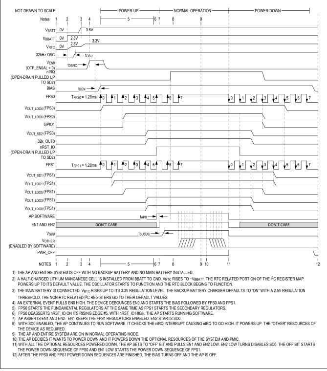
Figure 26. Application Processor Power-Up and Power-Down Timing
