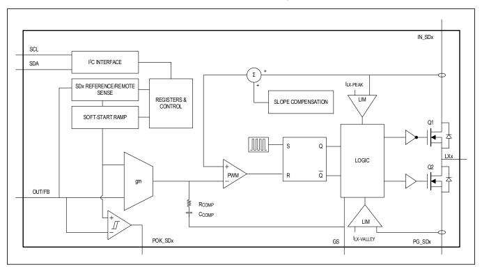
Figure 9. Buck Control Scheme Diagram
