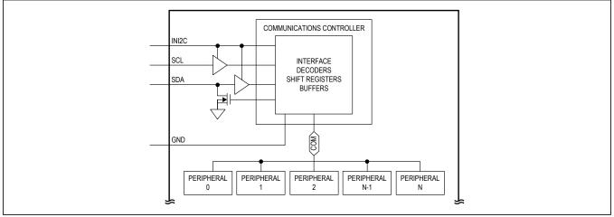
Figure 29. Functional Logic Diagram: Communications Controller
