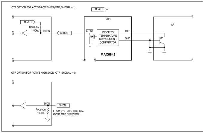
Figure 25. SHDN Simplified Input Stage: Active-High or Low
