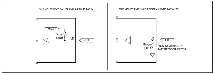
Figure 24. LID Simplied Input Stage: Active-High or Low
