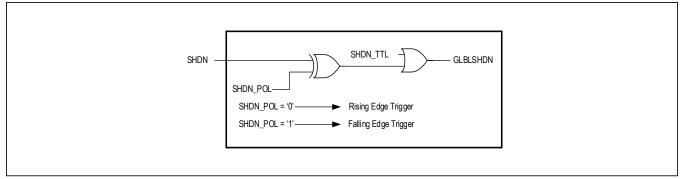
Figure 17. Functional Block Diagram for SHDN
