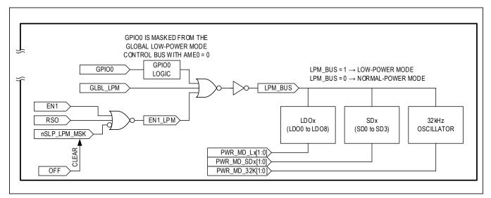
Figure 8. Simplified Logic for Global Low-Power Mode
