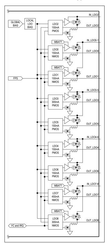
Figure 10. Linear Regulator Functional Diagram
