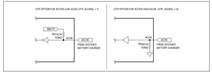
Figure 23. ACOK Simplified Input Stage: Active-High or Low
