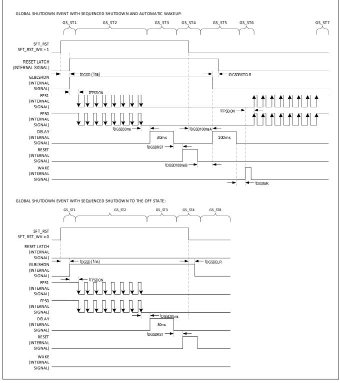
Figure 6. Simplified Timing Diagram for Global Shutdown
