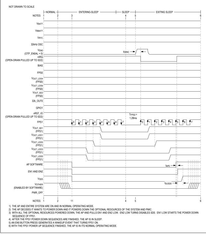
Figure 27. Application Processor Entering and Exiting Sleep Timing
