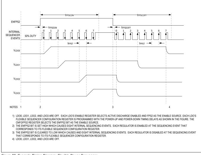
Figure 28. Example Timing Diagram: Flexible Power Sequencer
