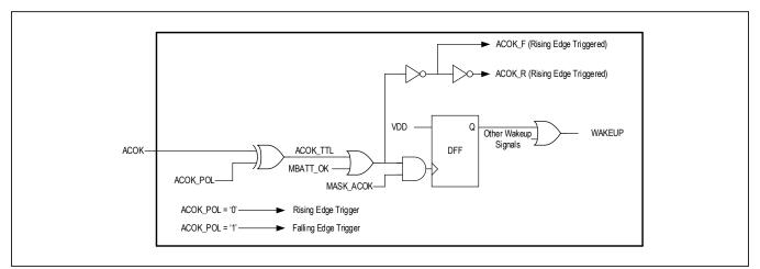
Figure 15. Functional Block Diagram for ACOK
