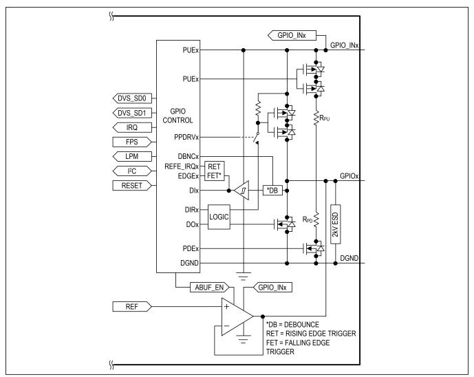
Figure 12. GPIO Simplified Block Diagram
