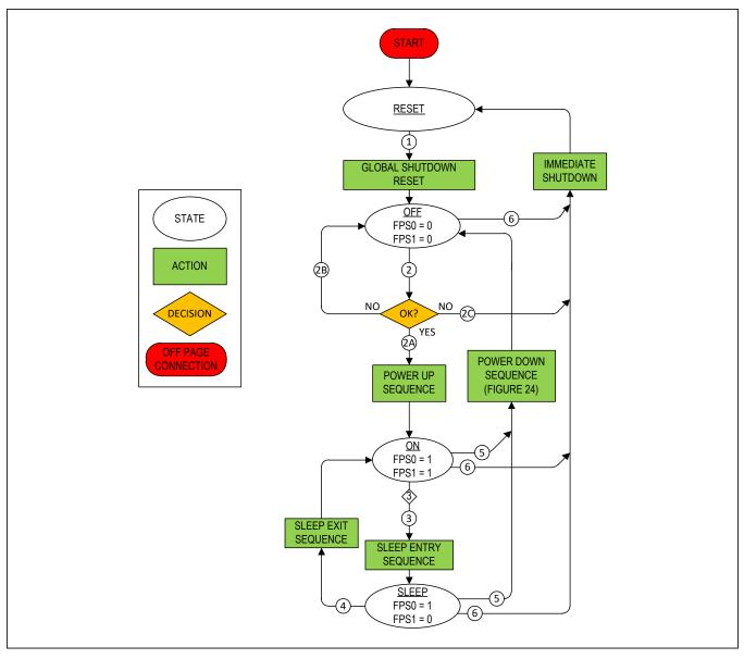
Figure 19. State Diagram: ON/OFF Controller
