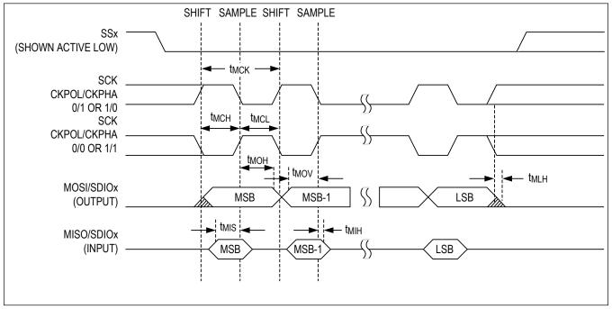
Figure 3. SPI Controller Mode Timing Diagram
