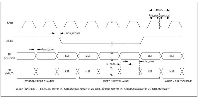
Figure 6. I<sup>2</sup>S Controller Timing Diagram
