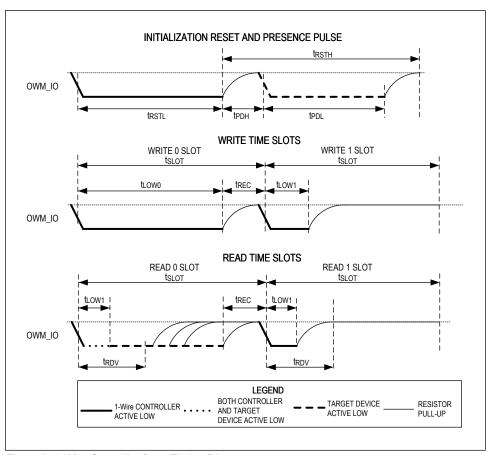
Figure 8. 1-Wire Controller Data Timing Diagram
