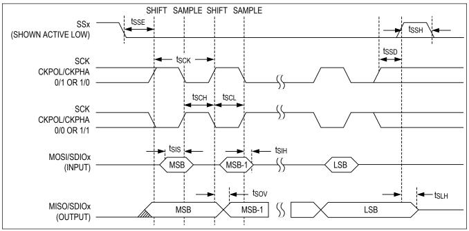
Figure 4. SPI Target Mode Timing Diagram
