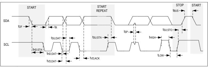
Figure 1. I<sup>2</sup>C Timing Diagram
