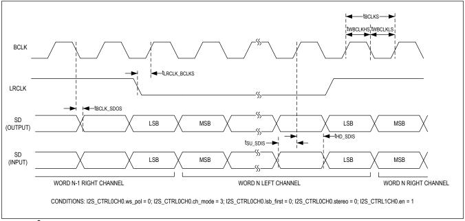
Figure 5. I<sup>2</sup>S Target ModeTiming Diagram
