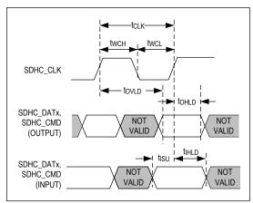
Figure 2. SD/SDIO/SDHC/MMC Timing Diagram
