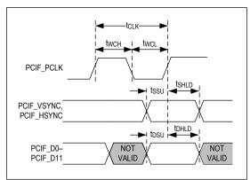
Figure 7. Parallel Camera Interface Timing Diagram
