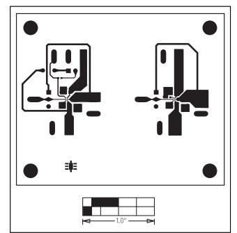
Figure 3. MAX8530/MAX8531 EV Kit PC Board Layout— Component Side
