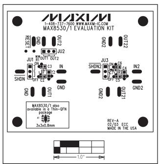
Figure 2. MAX8530/MAX8531 EV Kit Component Placement Guide—Component Side
