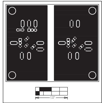
Figure 4. MAX8530/MAX8531 EV Kit PC Board Layout— Solder Side
