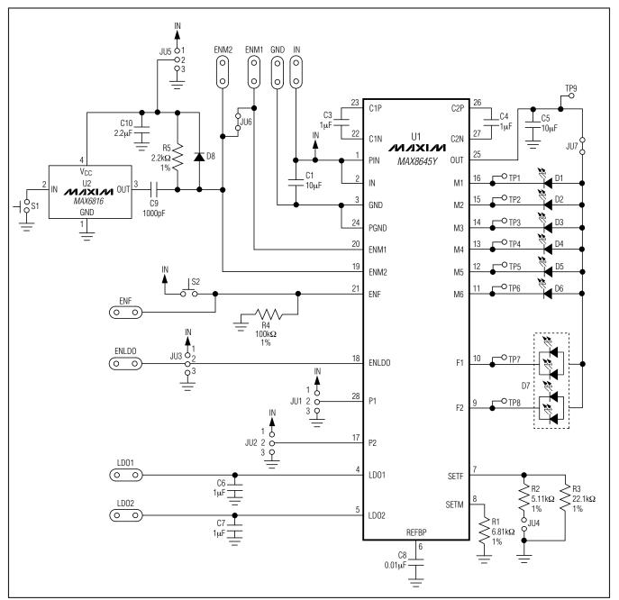
Figure 2. MAX8645Y EV Kit Schematic
