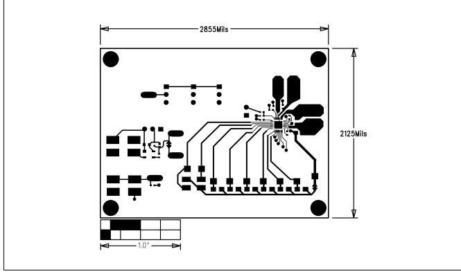
Figure 4. MAX8645Y EV Kit PCB Layout—Component Side
