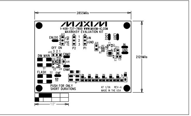
Figure 3. MAX8645Y EV Kit Component Placement Guide—Component Side
