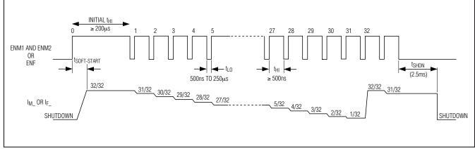
Figure 1. ENM\_ and ENF Timing Diagram
