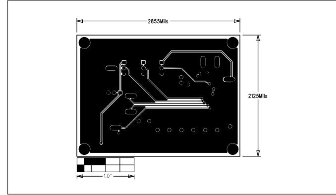
Figure 5. MAX8645Y EV Kit PCB Layout—Solder Side
