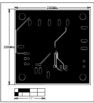
Figure 6. MAX8677A EV Kit PCB Layout—Layer 3
