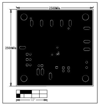
Figure 7. MAX8677A EV Kit PCB Layout—Solder Side
