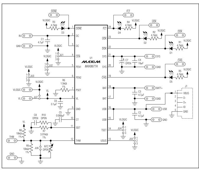
Figure 2. MAX8677A EV Kit Schematic
