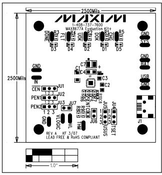
Figure 3. MAX8677A EV Kit Component Placement Guide—Component Side
