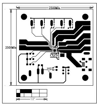
Figure 4. MAX8677A EV Kit PCB Layout—Component Side
