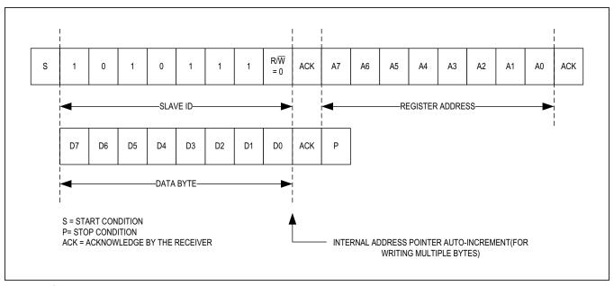
Figure 6. I<sup>2</sup>C Single Byte Write Transaction
