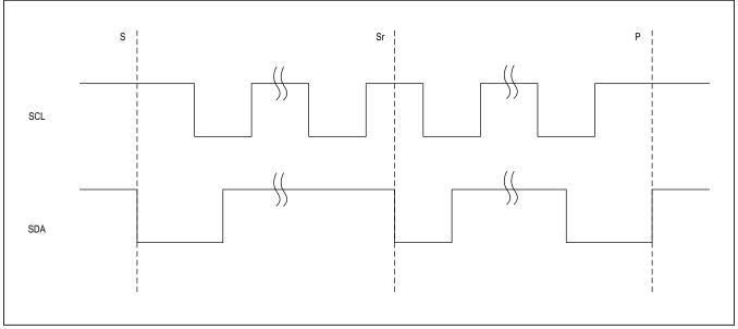
Figure 4: I<sup>2</sup>C START, STOP, and REPEATED START Conditions
