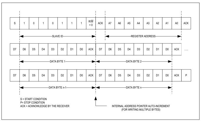
Figure 7. I<sup>2</sup>C Multi-Byte Write Transaction
