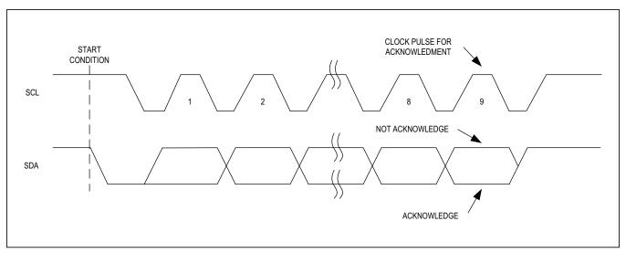
Figure 5. I<sup>2</sup>C Acknowledge Bit
