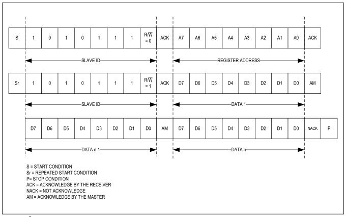
Figure 9. I<sup>2</sup>C Multi-Byte Read Transaction
