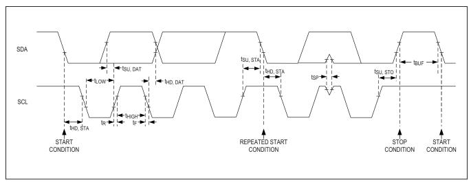
Figure 3. Detailed I<sup>2</sup>C Timing Diagram
