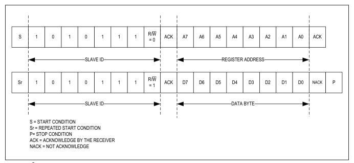
Figure 8. I<sup>2</sup>C Single Byte Read Transaction
