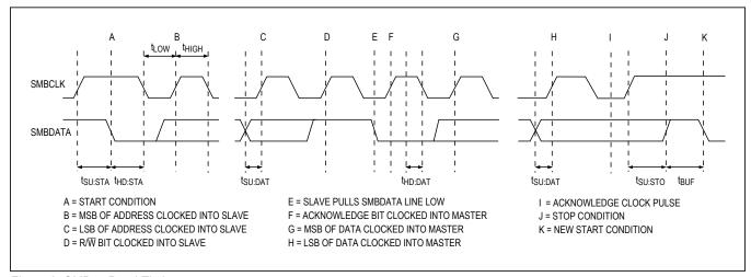
Figure 8. SMBus Read Timing
