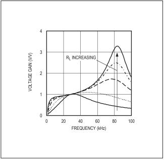
Figure 5. Frequency Response of the Resonant Tank
