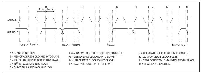
Figure 7. SMBus Write Timing
