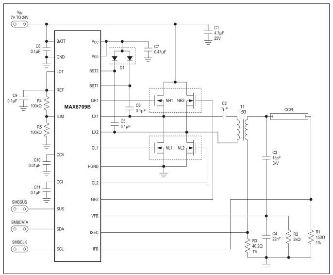
Figure 1. Typical Operating Circuit
