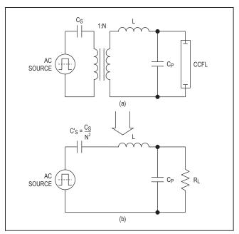
Figure 4. Equivalent Resonant Tank Circuit
