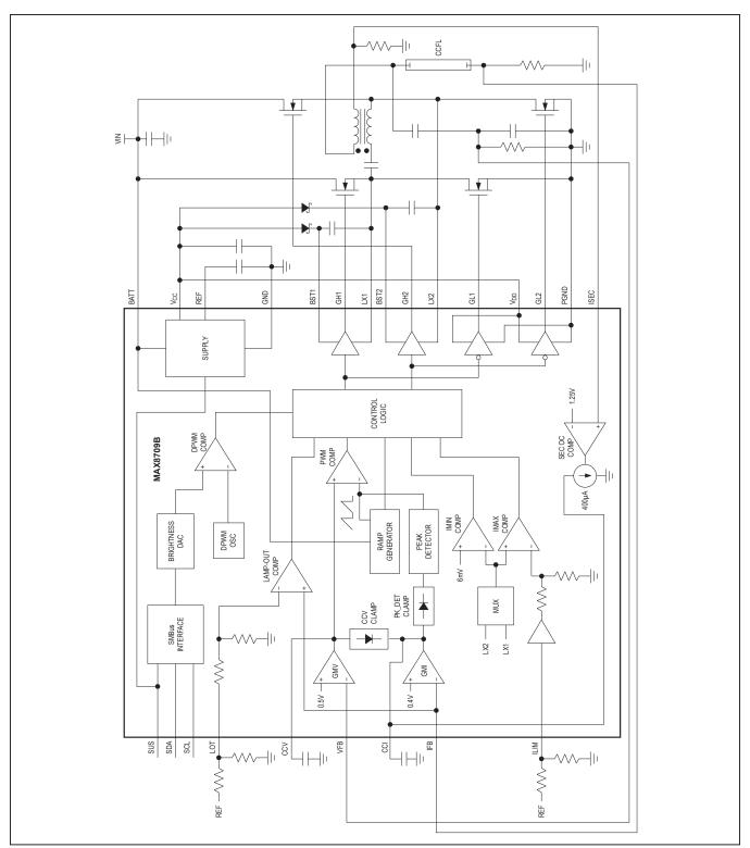
Figure 2. Functional Diagram
