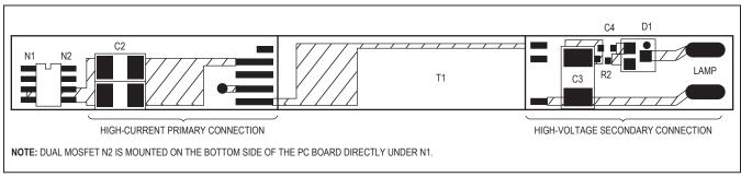
Figure 9. High-Voltage Components Layout Example
