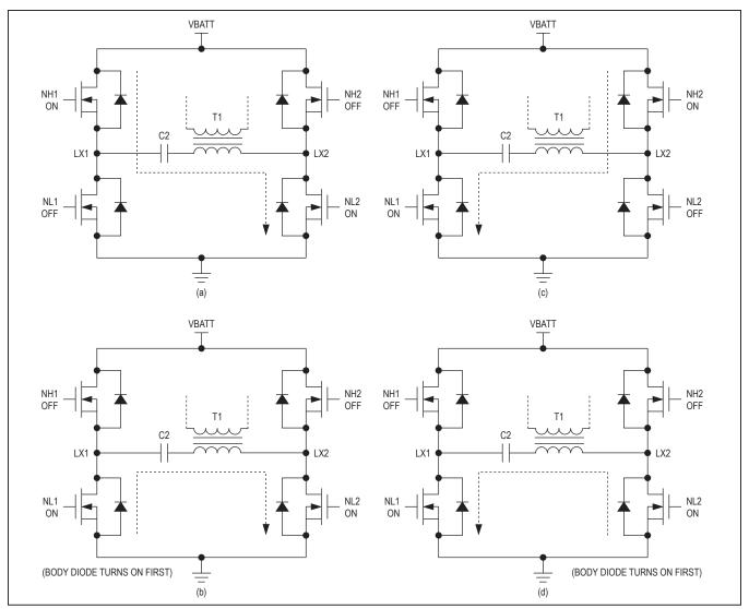
Figure 3. Resonant Operation
