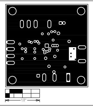
Figure 4. MAX8739 EV Kit PC Board Layout—GND Layer 2
