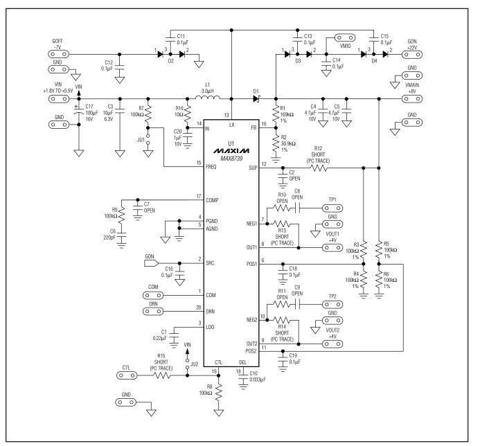
Figure 1. MAX8739 EV Kit Schematic
