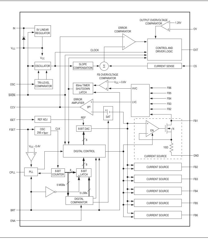
Figure 2. Control Circuit Block Diagram
