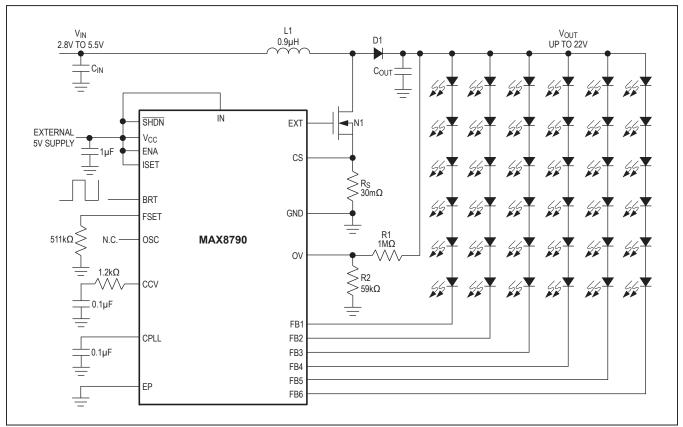
Figure 3. Low-Input-Voltage Application Circuit
