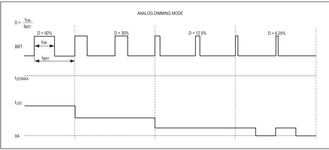
Figure 4. LED Current Control Using Analog Dimming Mode
