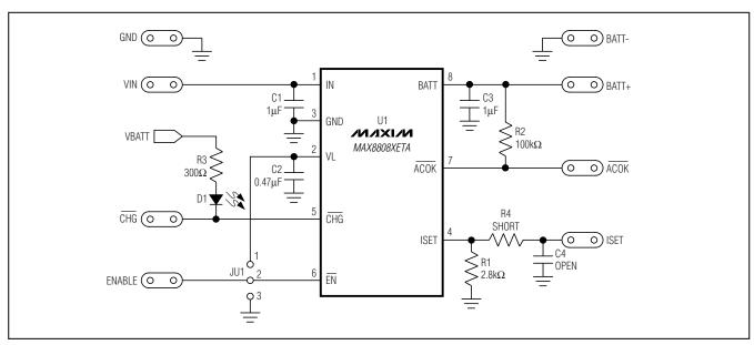
Figure 1. MAX8808 EV Kit Schematic
