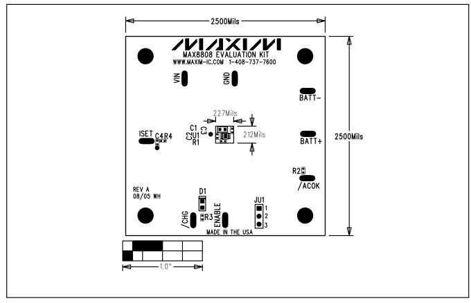
Figure 2. MAX8808 EV Kit Component Placement Guide—Component Side
