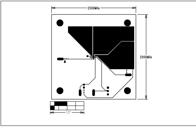
Figure 3. MAX8808 EV Kit PC Board Layout—Component Side
