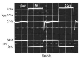
$V_{IN} = V_{OUT} + 0.1V$ ,  $I_{LOAD} = 0mA$  to 50mA,  $C_{IN} = 10\mu F$ , V<sub>OUT</sub> IS AC COUPLED
