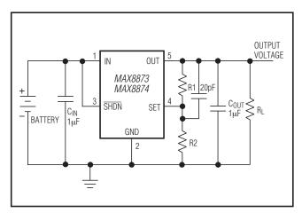
Figure 2. Adjustable Output Using External Feedback Resistors
