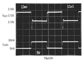
$I_{LOAD} = 0mA$  to 50mA,  $C_{IN} = 10 \mu F, \, V_{OUT} \, IS \, AC \, \, COUPLED$
