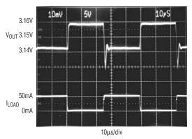
$V_{IN} = V_{OUT} + 0.2 V, \; I_{LOAD} = 0 mA \; to \; 50 mA, \; C_{IN} = 10 \mu F, \;$ V<sub>OUT</sub> IS AC COUPLED
