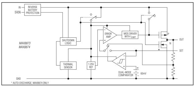
Figure 1. Functional Diagram
