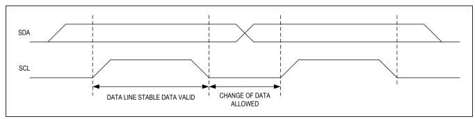
Figure 7. I<sup>2</sup>C Bit Transfer
