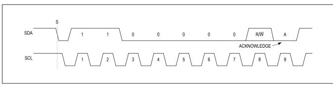
Figure 9. Slave Address Byte Example
