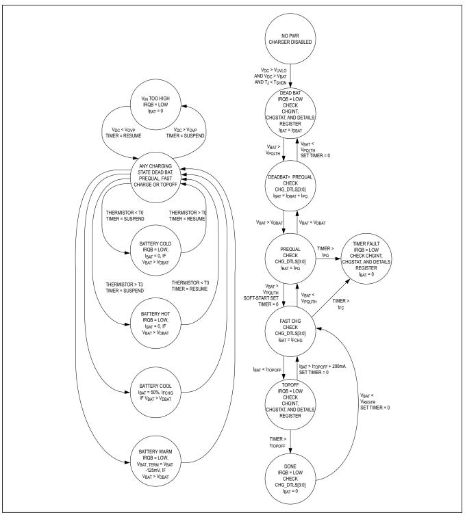
Figure 3. Functional State Diagram
