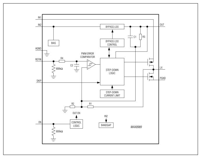
Figure 1. Functional Diagram
