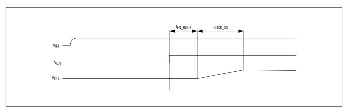
Figure 2. Power-Up Timing
