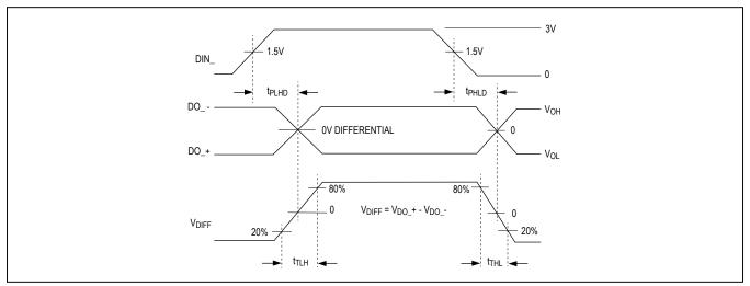
Figure 3. Transmitter Propagation Delay and Transition Time Waveforms
