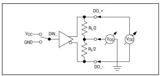
Figure 1. LVDS Transmitter VOD and VOS Test Circuit
