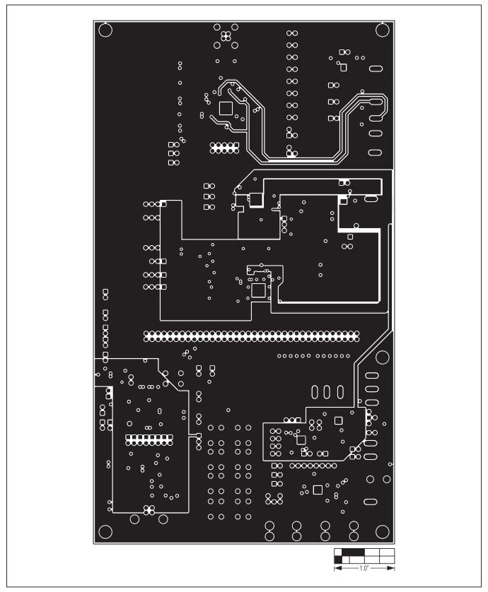
Figure 14. MAX9266 EV Kit PCB Layout—Power Layer 3
