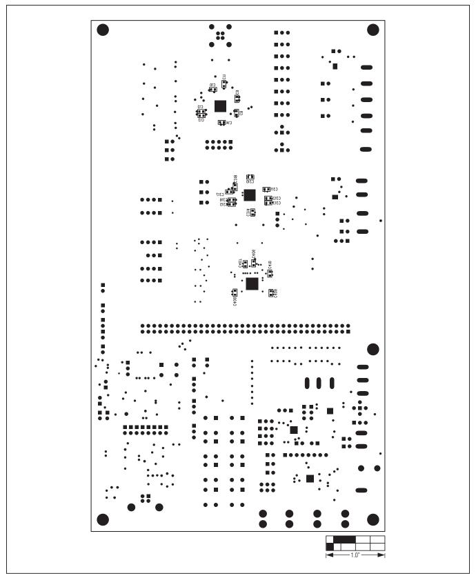
Figure 11. MAX9266 EV Kit Component Placement Guide—Solder Side
