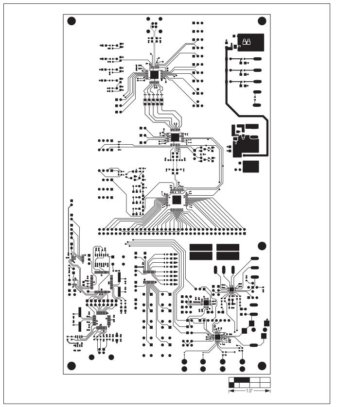
Figure 12. MAX9266 EV Kit PCB Layout—Component Side
