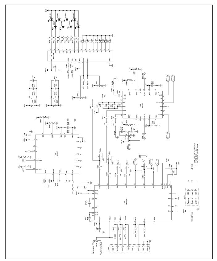
Figure 9c. MAX9266 EV Kit Schematic (Sheet 3 of 5)
