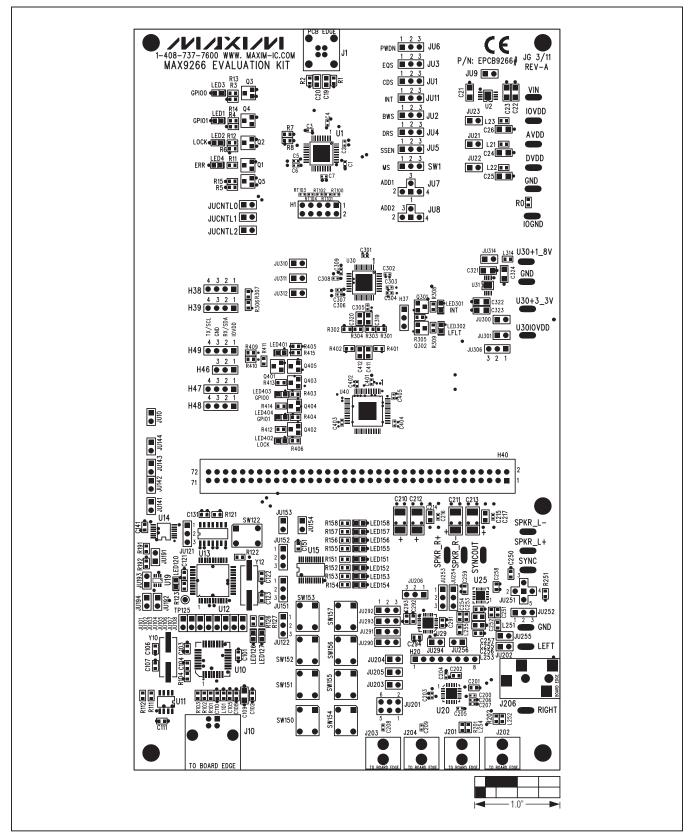
Figure 10. MAX9266 EV Kit Component Placement Guide—Component Side
