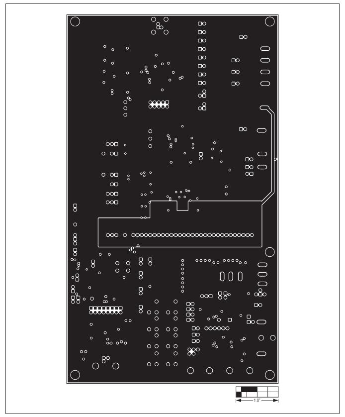
Figure 13. MAX9266 EV Kit PCB Layout—Ground Layer 2
