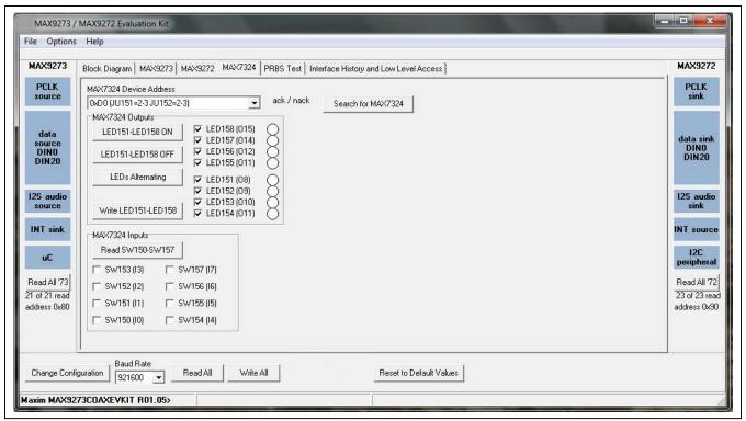
Figure 4. MAX9273/MAX9272 EV Kit Software Main Window (MAX7324 Tab)
