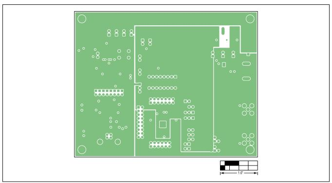
Figure 14. MAX9273 Coax EV Kit PCB Layout—Power Layer 3
