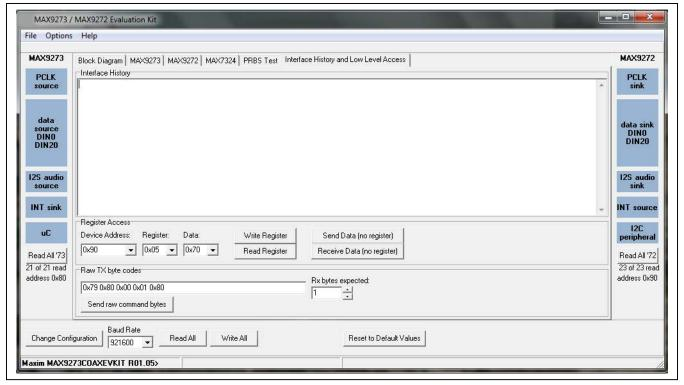
Figure 7. MAX9273/MAX9272 EV Kit Software Connect Window
