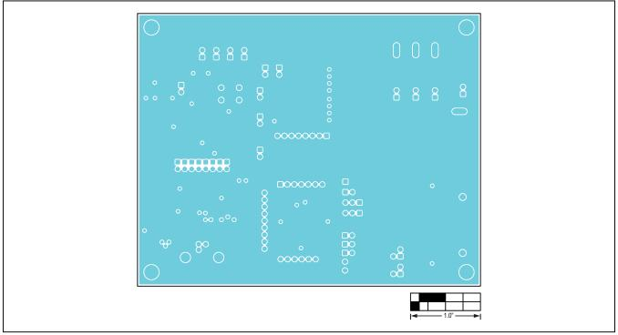
Figure 13. MAX9273 Coax EV Kit PCB Layout—Ground Layer 2
