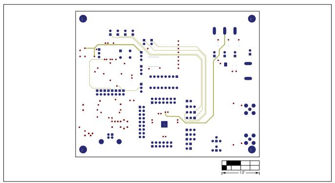
Figure 15. MAX9273 Coax EV Kit PCB Layout—Solder Side
