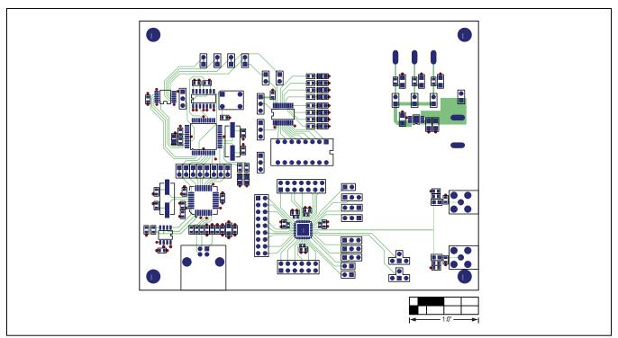
Figure 12. MAX9273 Coax EV Kit PCB Layout—Component Side
