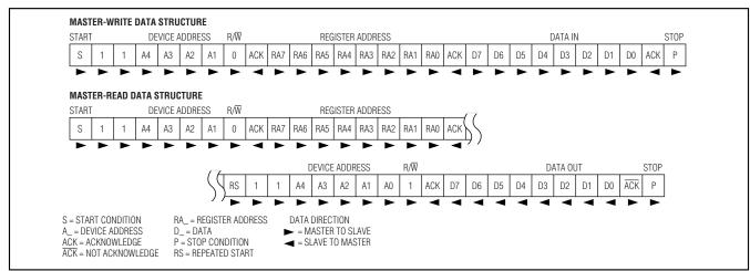
Figure 4. I<sup>2</sup>C Interface Data Structure
