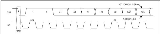
Figure 3. I<sup>2</sup>C Address and Acknowledge
