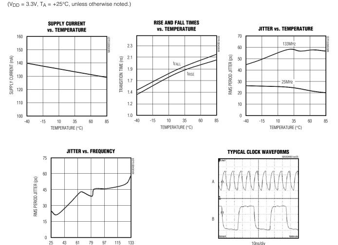
10ns/div A: 100MHz. 100mV/div B: 25MHz, 100mV/div
