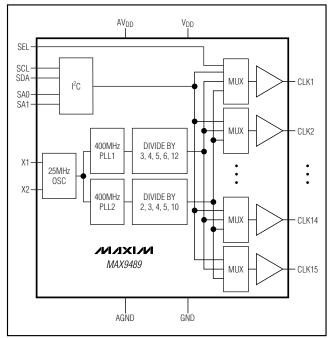
Figure 1. MAX9489 Functional Diagram
