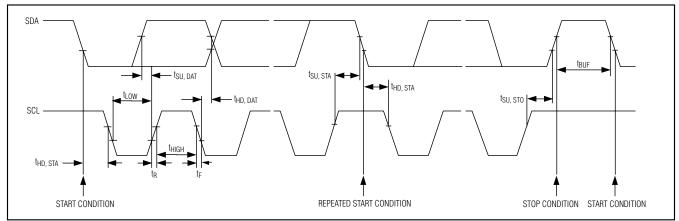
Figure 2. Serial Interface Timing
