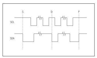
Figure 2. START, STOP, and REPEATED START Conditions
