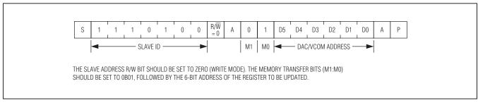
Figure 9. Updating a Single DAC Register with MTP Memory Data (Single Acquire Command)
