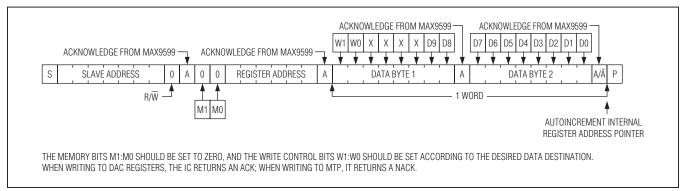
Figure 4. Writing a Word of Data to the IC's DAC or MTP Registers
