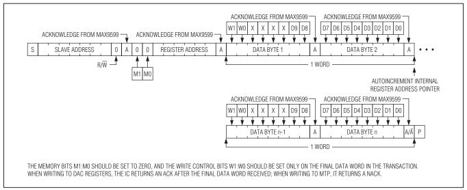
Figure 5. Writing Multiple Words of Data to the IC's DAC or MTP Registers
