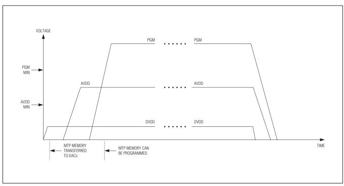
Figure 10. Conventional Power-Up and Power-Down Sequence
