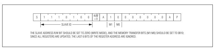
Figure 8. Updating All DAC Registers from MTP Memory Data (General Acquire Command)
