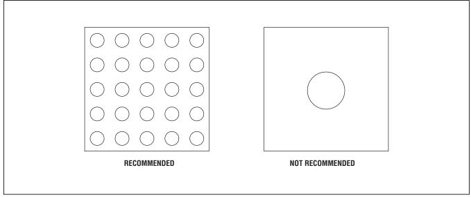
Figure 11. Multiple Small Vias are Recommended over a Single Large Via in the PCB Layout
