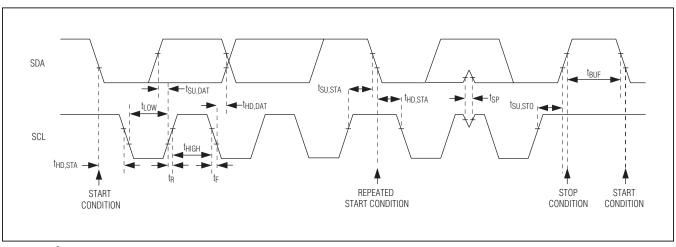
Figure 1. I<sup>2</sup>C Interface Timing Diagram
