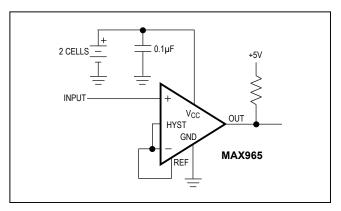
Figure 6. 2-Cell to TTL Logic-Level Translator
