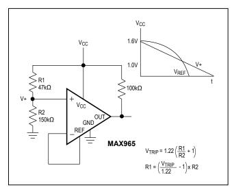
Figure 1. Operation below 1.6V
