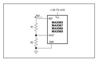
Figure 3. Programming the HYST Pin
