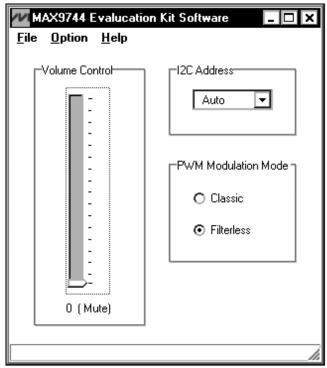
Figure 1. MAX9744 EV Kit Software GUI Window
