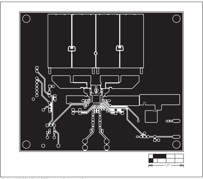
Figure 4. MAX9744 EV Kit PCB Layout—Component Side
