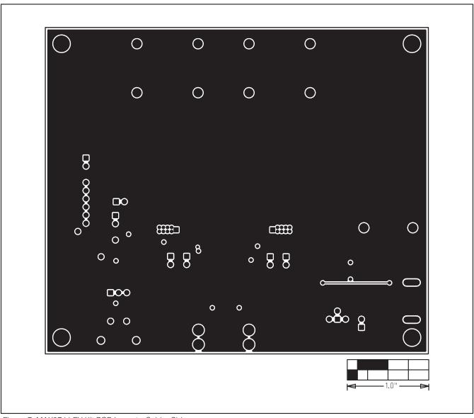
Figure 7. MAX9744 EV Kit PCB Layout—Solder Side
