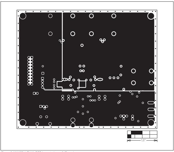
Figure 6. MAX9744 EV Kit PCB Layout—Layer 3 (Power)
