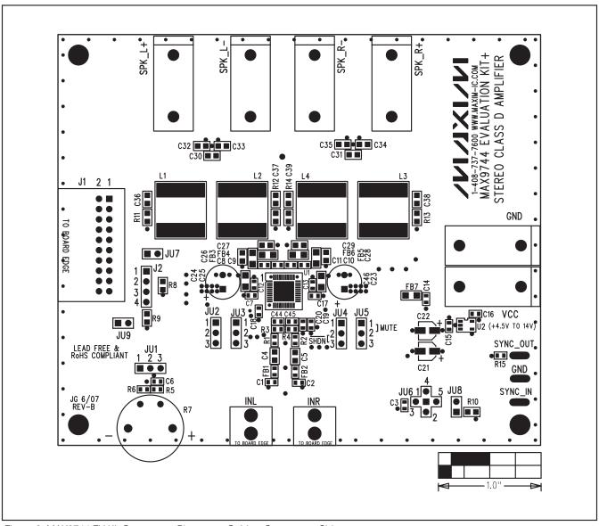
Figure 3. MAX9744 EV Kit Component Placement Guide—Component Side
