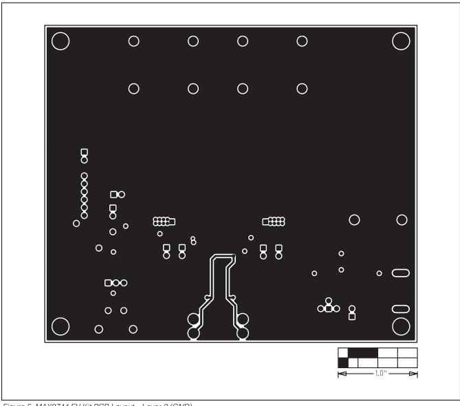
Figure 5. MAX9744 EV Kit PCB Layout—Layer 2 (GND)
