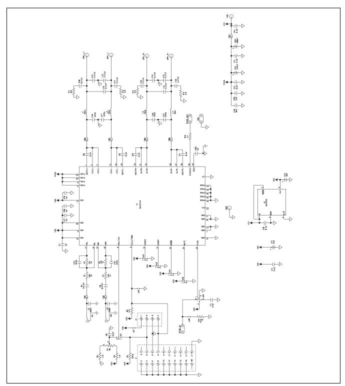
Figure 2. MAX9744 EV Kit Schematic
