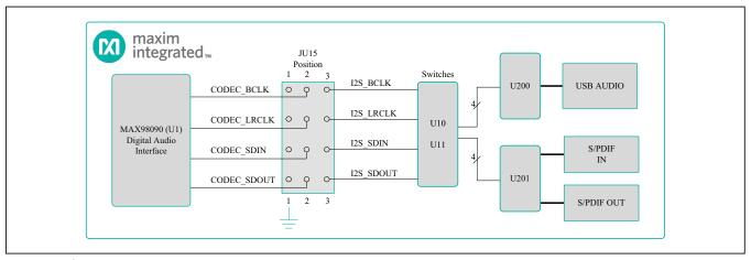
Figure 13. I<sup>2</sup>S Routing
