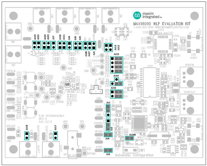
Figure 2. Default Shunt Configuration
