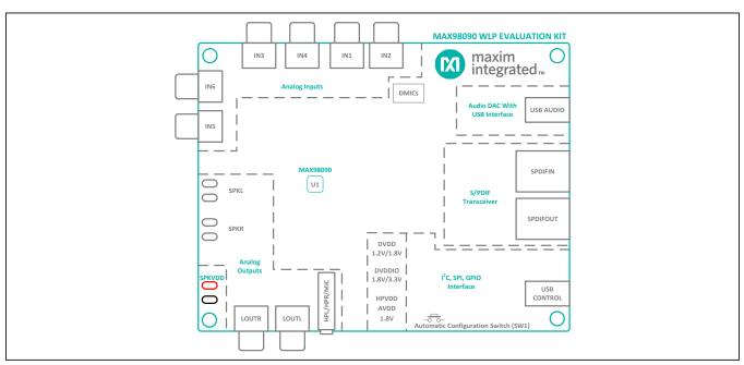
Figure 1. Simplified EV Kit Block Diagram
