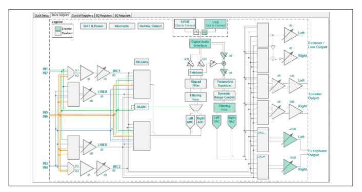
Figure 7. MAX98090 Software Block Diagram
