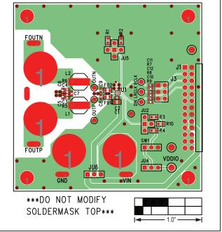
MAX98357 DEV Board PCB Layout—Component Side
