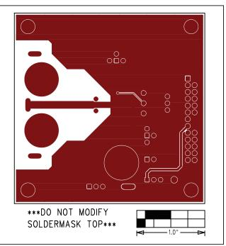
MAX98357 DEV Board PCB Layout—Solder Side
