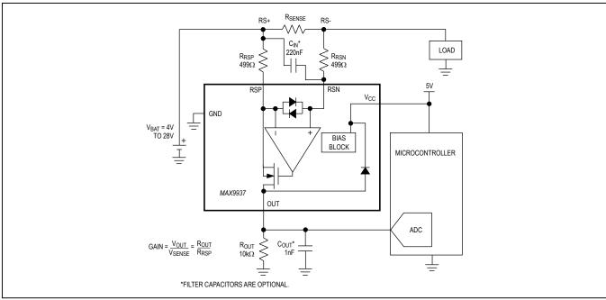
Figure 1. Typical Application Circuit with Optional External Filtering
