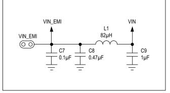
Figure 1. EMI Filter Components
