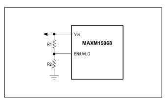
Figure 1. Adjustable EN/UVLO Network
