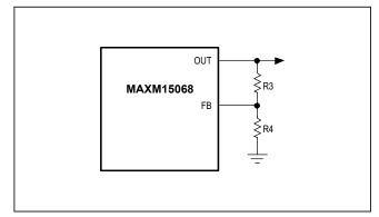
Figure 2. Setting the Output Voltage
