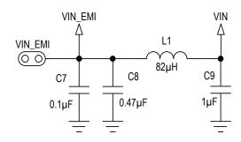
Figure 1. EMI Filter Components
