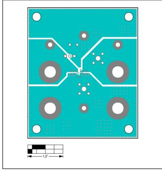
MAXM17225 EV Kit PCB Layout—Top View
