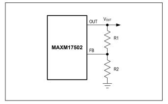
Figure 1: Adjusting Output Voltage
