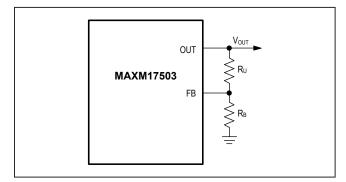
Figure 1. Adjustable Output Voltage
