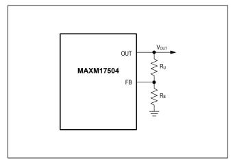
Figure 1. Adjustable Output Voltage
