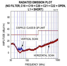
FREQUENCY (MHz) CONDITIONS : VIN = 24V, VOUT = 5V, IOUT = 4A FROM : MAXM17536EVKIT#
