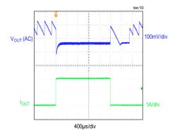
LOAD TRANSIENT (V<sub>IN</sub> = 24V, V<sub>OUT</sub> = 5V, I<sub>OUT</sub> = 25mA TO 2A, DCM MODE)
