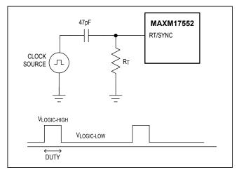
Figure 1. Synchronization to an External Clock
