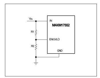
Figure 2. Adjustable EN/UVLO Network
