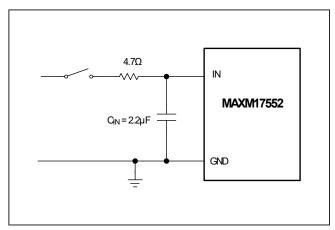
Figure 4. Circuit for Transient Protection
