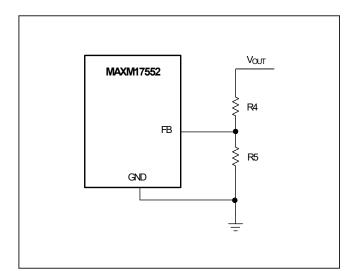
Figure 3 Circuit for Setting the Output Voltage.
