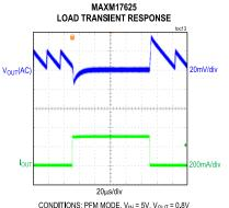
CONDITIONS: PFM MODE,  $\rm V_{IN}$  = 5V,  $\rm V_{OUT}$  = 0.8V LOAD STEP BETWEEN 5mA TO 300mA
