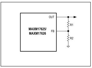
Figure 2. Setting the Output Voltage
