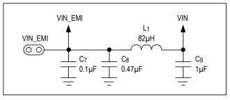
Figure 1. EMI Filter Components
