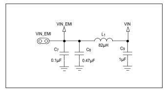
Figure 1. EMI Filter Components
