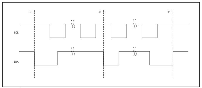
Figure 10. I<sup>2</sup>C START, STOP, and REPEATED START Conditions
