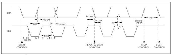
Figure 9. Detailed I<sup>2</sup>C Timing Diagram
