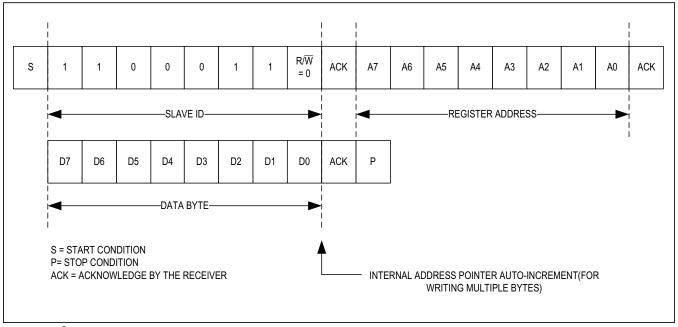
Figure 12. I<sup>2</sup>C Single Byte Write Transaction
