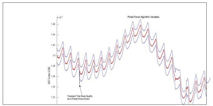
Figure 7. Picket Fences Variables In A PPG Waveform
