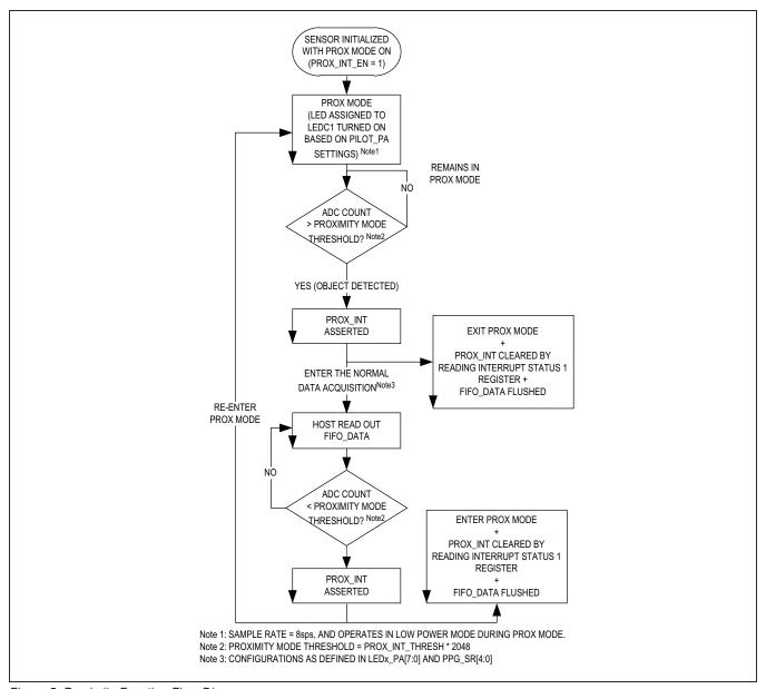
Figure 5. Proximity Function Flow Diagram
