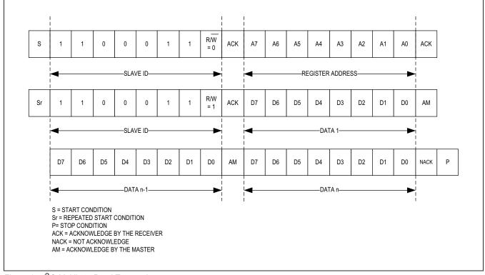
Figure 15. I<sup>2</sup>C Multibyte Read Transaction
