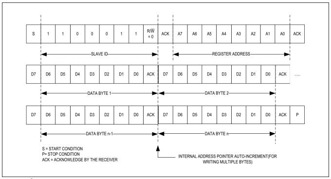
Figure 13. I<sup>2</sup>C Multi-Byte Write Transaction
