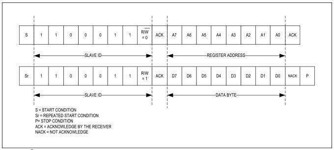
Figure 14. I<sup>2</sup>C Single Byte Read Transaction
