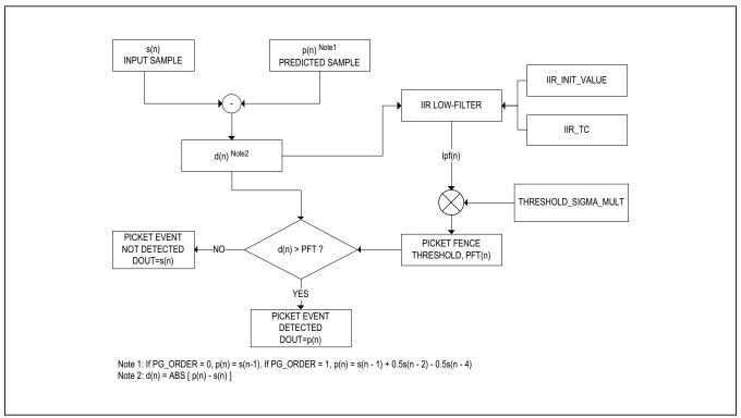
Figure 6. Picket Fence Function Flow
