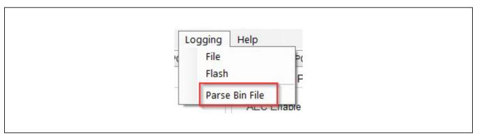
Figure 19. MAXM86161 EV System GUI: Bin-to-CSV Data File Format Conversion Option
