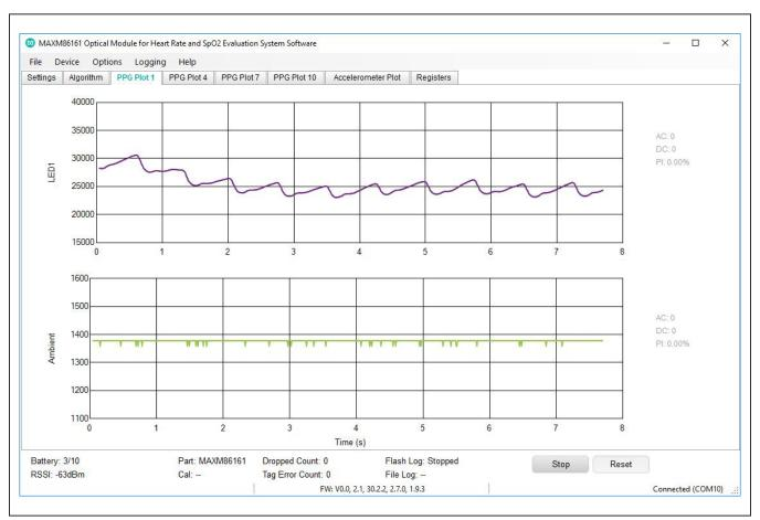
Figure 13. MAXM86161 EV System GUI (PPG Plots)
