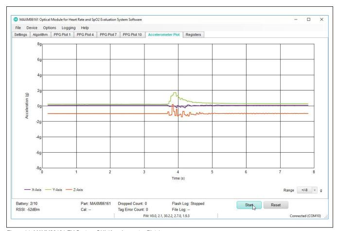
Figure 14. MAXM86161 EV System GUI (Accelerometer Plots)
