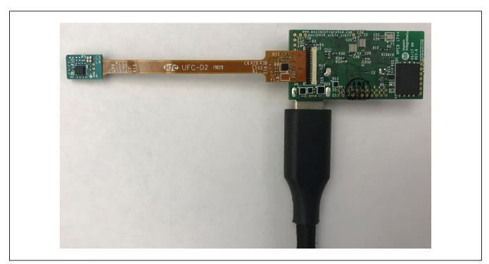
Figure 3. Hardware Setup (MAXM86161 EV System Sensor PCB)
