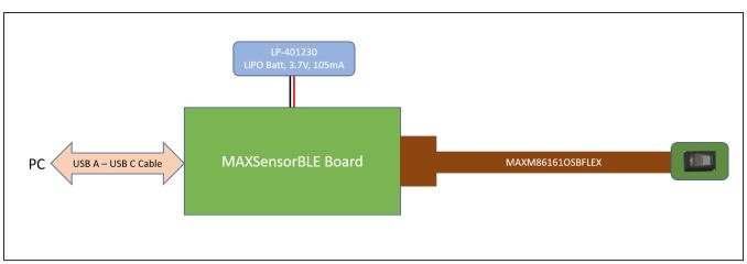
Figure 1. MAXM86161 EV System Block Diagram
