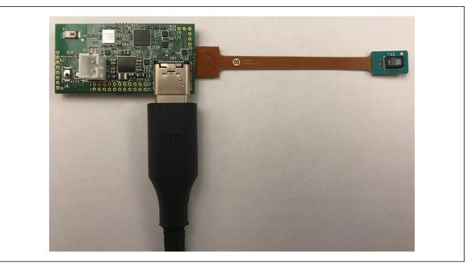
Figure 2. Hardware Setup (MAXM86161 EV System Micro PCB)
