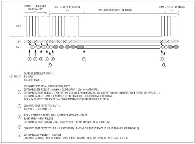
Figure 6. Receive Burst-Count Example
