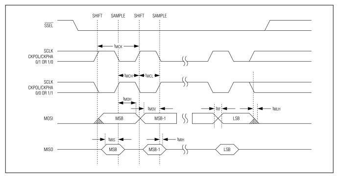
Figure 7. SPI Master Communication Timing
