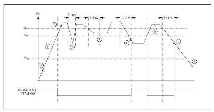
Figure 10. Power-Fail Detection During Normal Operation
