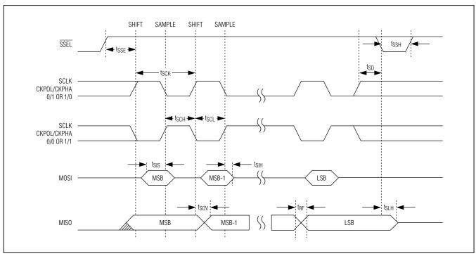
Figure 8. SPI Slave Communication Timing
