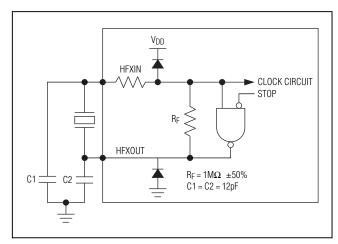
Figure 9. On-Chip Oscillator
