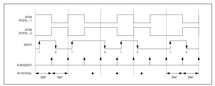
Figure 4. External IRTXM (Modulator) Output
