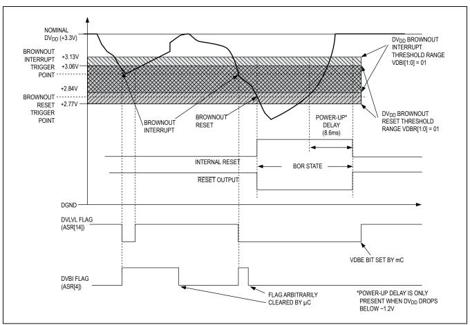
Figure 5. DVDD Brownout Interrupt Detection
