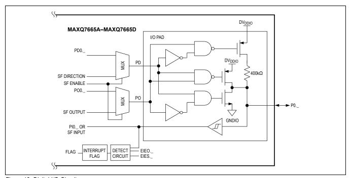
Figure 13. Digital I/O Circuitry
