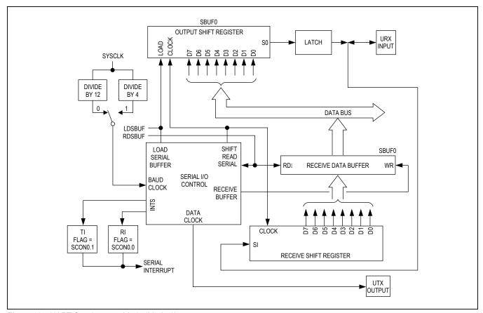
Figure 11a. UART Synchronous Mode (Mode 0)
