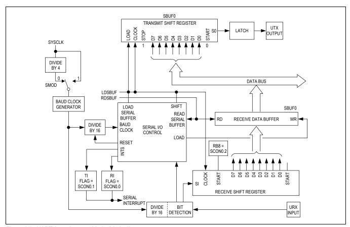
Figure 11b. UART Asynchronous Mode (Mode 1)
