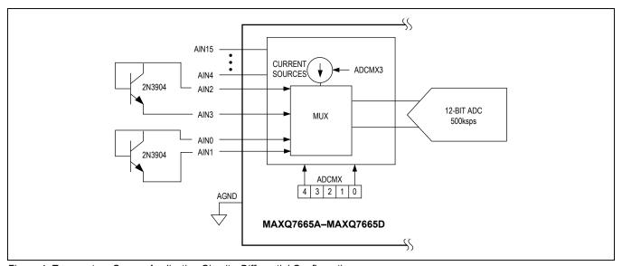
Figure 4. Temperature-Sensor Application Circuit—Differential Configuration
