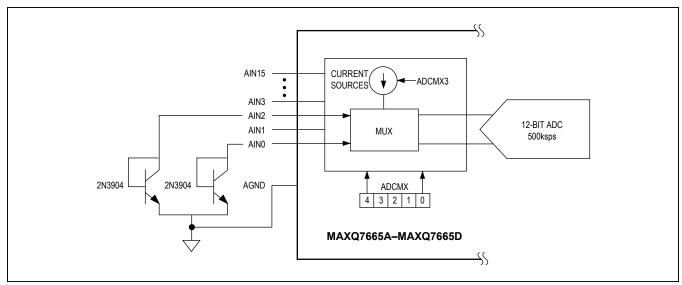
Figure 3. Temperature-Sensor Application Circuit—Single-Ended Configuration
