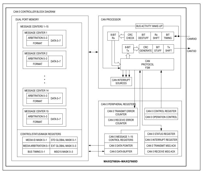
Figure 10. CAN 0 Controller Block Diagram
