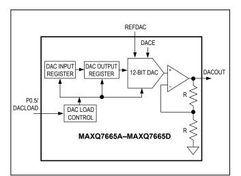
Figure 2. Simplified DAC Diagram
