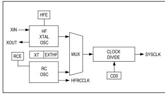
Figure 6. High-Frequency and RC Oscillator Block Diagram
