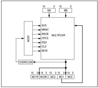
Figure 9. 16-Bit Hardware Multiplier Functional Diagram
