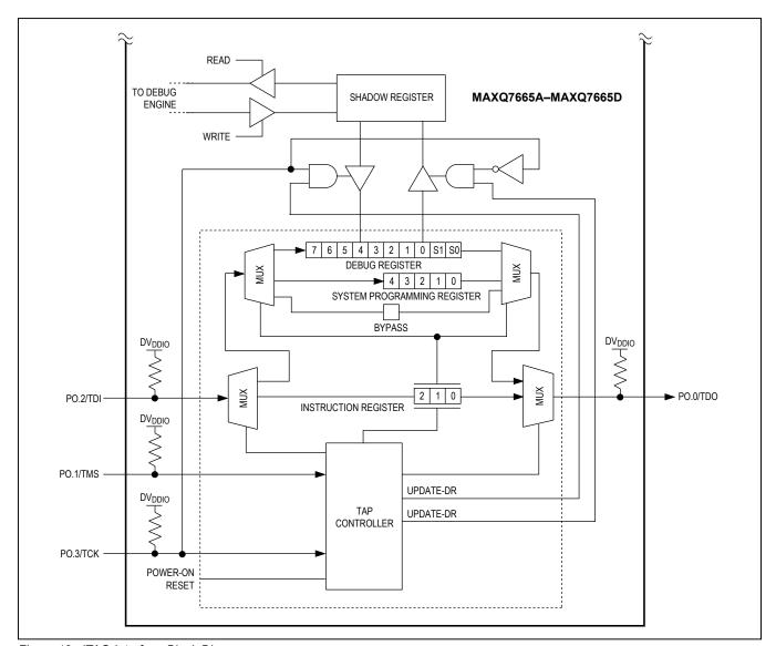
Figure 12. JTAG Interface Block Diagram
