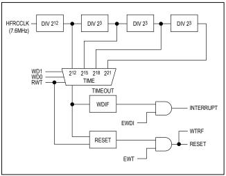
Figure 7. Watchdog Functional Diagram
