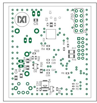
Figure 5. MAXQ7667 Component Placement Guide—Solder Side
