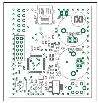
Figure 4. MAXQ7667 Component Placement Guide— Component Side
