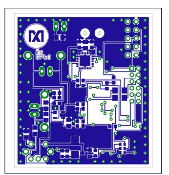
Figure 7. MAXQ7667 PCB Layout—Solder Side
