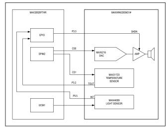
Figure 1. Block Diagram
