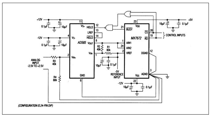
Figure 13. MX7672—AD585 Sample-and-Hold Interface
