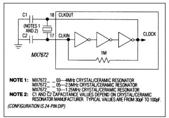
Figure 6. MX7672 Internal Clock Circuit
