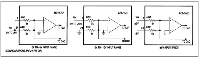
Figure 15. Analog Input Range Configurations
