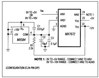
Figure 16. Unipolar Operation Using an MX584 Reference
