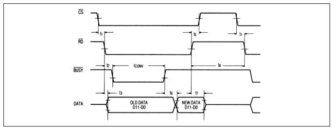
Figure 9. Slow-Memory Mode Timing Diagram
