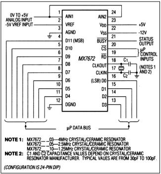
Figure 3. MX7672 Operational Diagram
