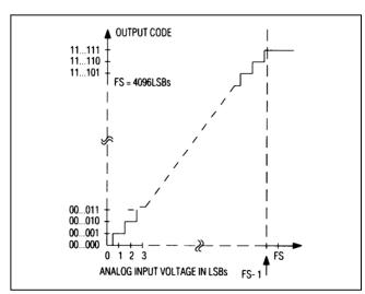
Figure 17. MX7672 Ideal Unipolar Transfer Function
