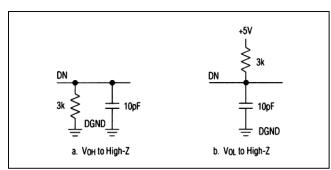
Figure 2. Load Circuits for Bus-Relinquish Time
