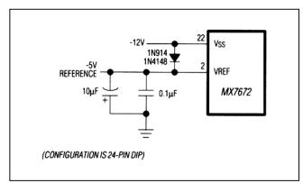
Figure 12. V<sub>REF</sub>/V<sub>SS</sub> Diode Clamp (See Reference Input section)
