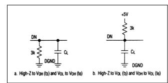
Figure 1. Load Circuits for Access Time
