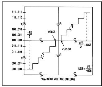
Figure 20. Ideal Input/Output Transfer Characteristic for Bipolar Operation
