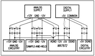
Figure 11. Power-Supply Grounding Practice
