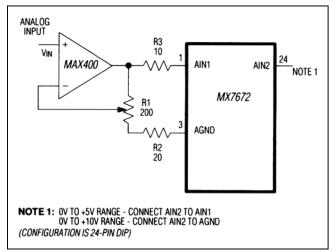
Figure 18. Unipolar Operation with Gain Adjust
