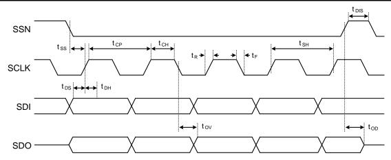
Use of the SPI is optional as SC1889 is capable of fully autonomous operation. Use of the SPI interface offers the user access to certain monitoring and diagnostic functions, as well as other planned advanced features. The SPI bus interface is also used to program the internal EEPROM, allowing changes to the operating frequency range, field upgrades, and firmware updates.
