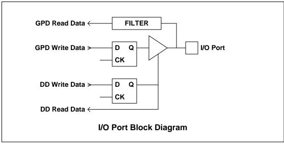
Figure 4-1. I/O Port Block Diagram
