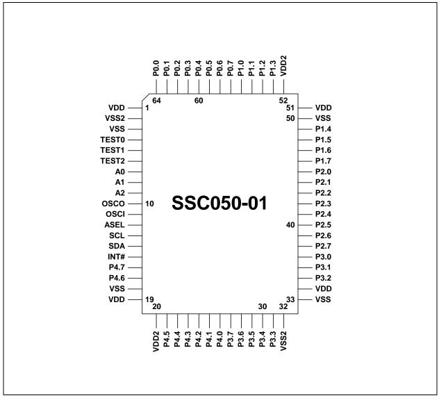
Figure 3-2. Pinout Diagram
