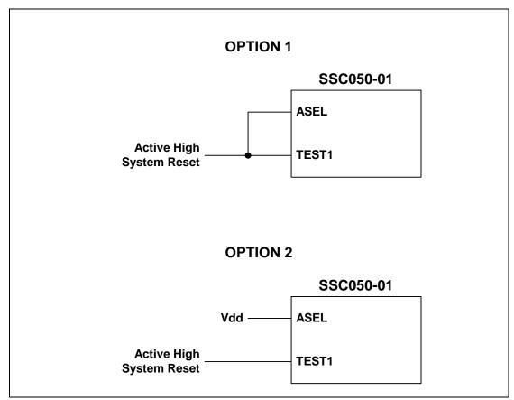
Figure 5-5. External Reset Circuit Options
