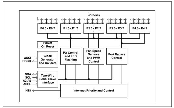
Figure 1-1. Chip Block Diagram
