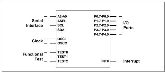
Figure 3-1. Functional Signal Grouping
