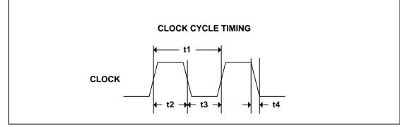
Figure 5-1. Clock Cycle Timing
