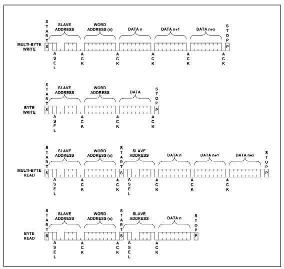
Figure 5-3. Two-Wire Serial Interface Operation
